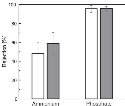
Fig. 2. Rejection of ammonium and phosphate ions using the surrogate AnMBR effluent.
