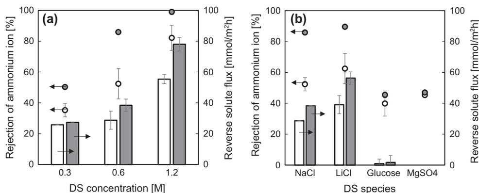
Fig. 5. Relationship between rejection of ammonium ions and reverse solute flux: (a) different DS concentrations and (b) different solute of DS species.
