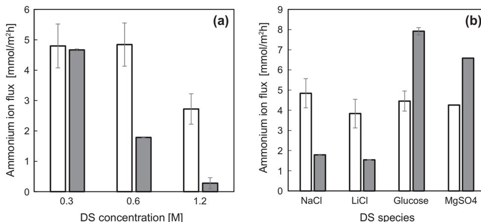
Fig. 6. Comparison of ammonium ion flux: (a) different DS concentrations and (b) different solute of DS species. Notes: 30 mg-N/L NH<sub>4</sub>Cl solution was used as the FS. White bars represent the result in AL-FS and gray bars represent the result in AL-DS.
