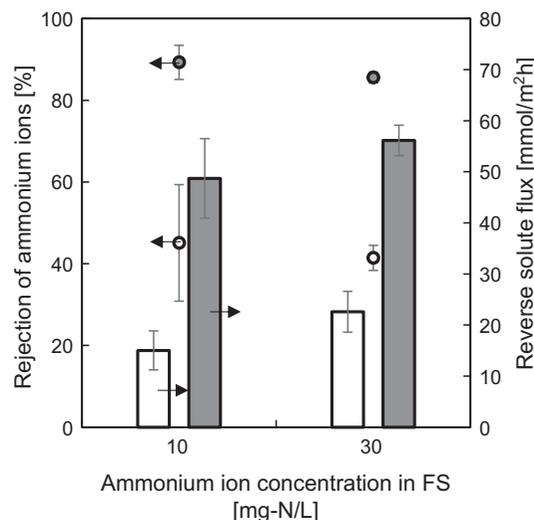
Fig. 3. Rejection of ammonium ions and reverse solute flux at different FS concentrations.
