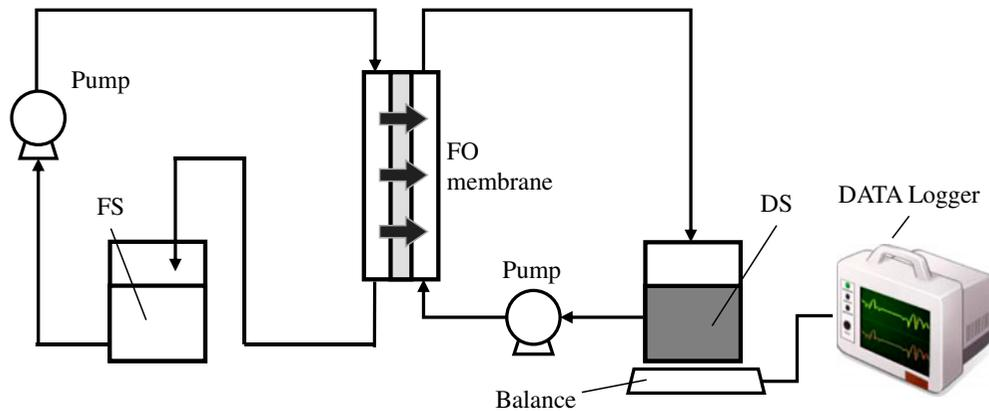
Fig. 1. Schematic representation of the lab-scale FO filtration unit.
