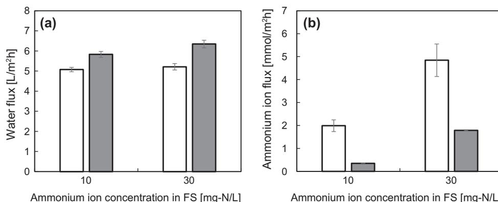
Fig. 4. Water flux and ammonium ion flux at different FS concentration (DS: 0.6 M NaCl); (a) comparison of water flux and (b) comparison of ammonium ion flux.
