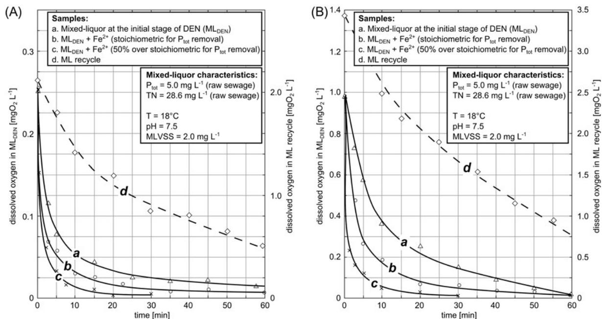
Fig. 2. Trend of DO in the preliminary batch tests carried out on ML samples collected simultaneously in the initial stage of denitrification (ML<sub>DEN</sub>) and in the mixed liquor recycle (ML<sub>recycle</sub>): cases with the lowest (A) and the highest (B) initial DO content.
