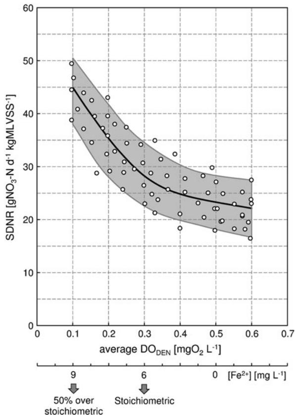
Fig. 4. SDNR as function of the average DO in the anoxic pre-denitrification tank (average  $DO_{DEN}$ ) at  $F:M_{DEN} = 0.3 \text{ kgBOD}_5 \text{ kgMLVSS}^{-1} \text{ d}^{-1}$  (temperature  $T = 18^\circ\text{C}$ ). The additional x-axis shows the concentration of the  $\text{Fe}^{2+}$  dosage. The continuous line and the shaded area represent the mean value and the 95% confidence limit, respectively.
