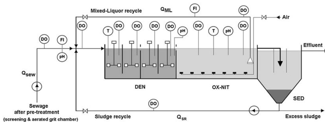
Fig. 1. Scheme of the pilot plant.
