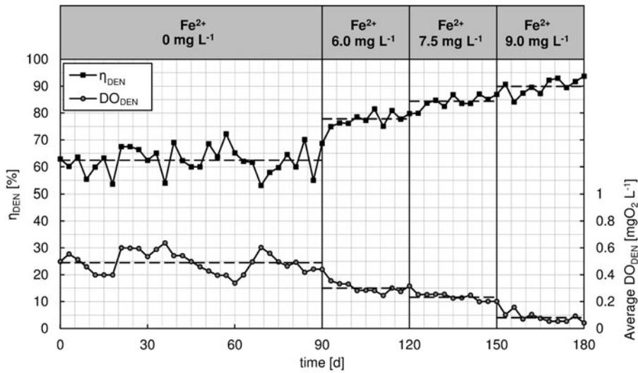
Fig. 3. Denitrification removal efficiency ( $\eta_{DEN}$ ) as function of the average DO content in the denitrification reactor (average  $DO_{DEN}$ ) during the four steps of the experimental period on the pilot plant. Dotted lines represent the mean values of  $\eta_{DEN}$  and  $DO_{DEN}$  in each experimental step.
