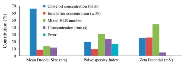
Fig. 4. Results of ANOVA for test series, contribution of each factor on the performance indicators.
