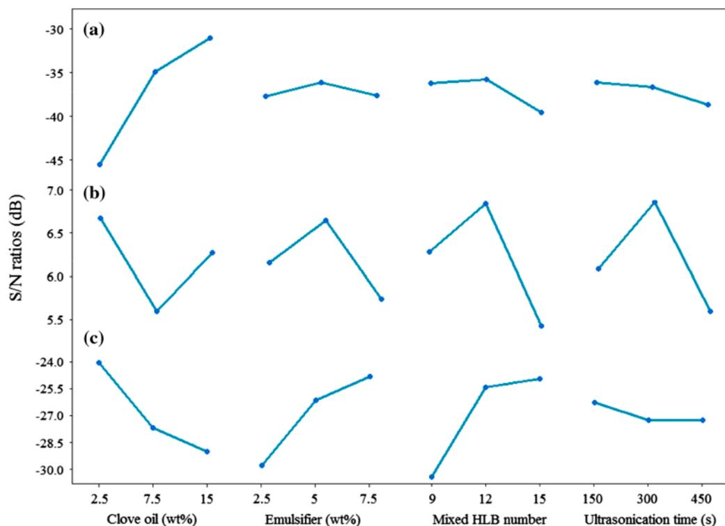
Fig. 3. S/N ratio graphs for (a) mean droplet size (nm), (b) PDI, and (c) zeta potential (mV).
