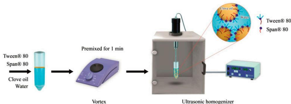
Fig. 2. Schematic diagram of the experimental set up for preparation of clove oil nanoemulsion.
