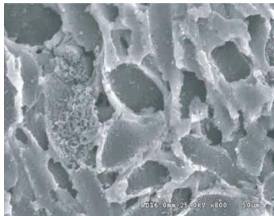
Fig. 1. Scanning electron microscope (SEM) photos of activated carbon type NP-5.
