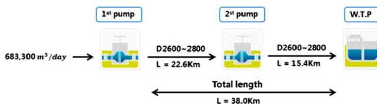
Fig. 1. Diagram of piping system.
