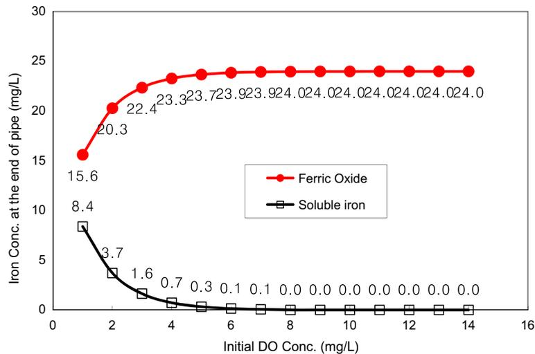
Fig. 4. Effect of DO on iron oxidation.
