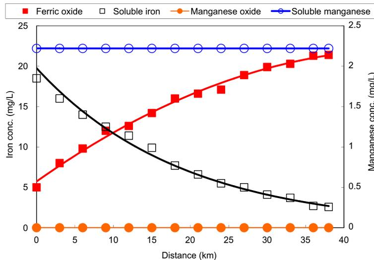
Fig. 2. Behaviors of iron and manganese with transport distance through pipe (modeled by EPANET-MSX).
