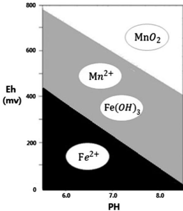
Fig. 3. States of iron and manganese with different Eh and pH (adapted from Hallberg et al. [13]).
