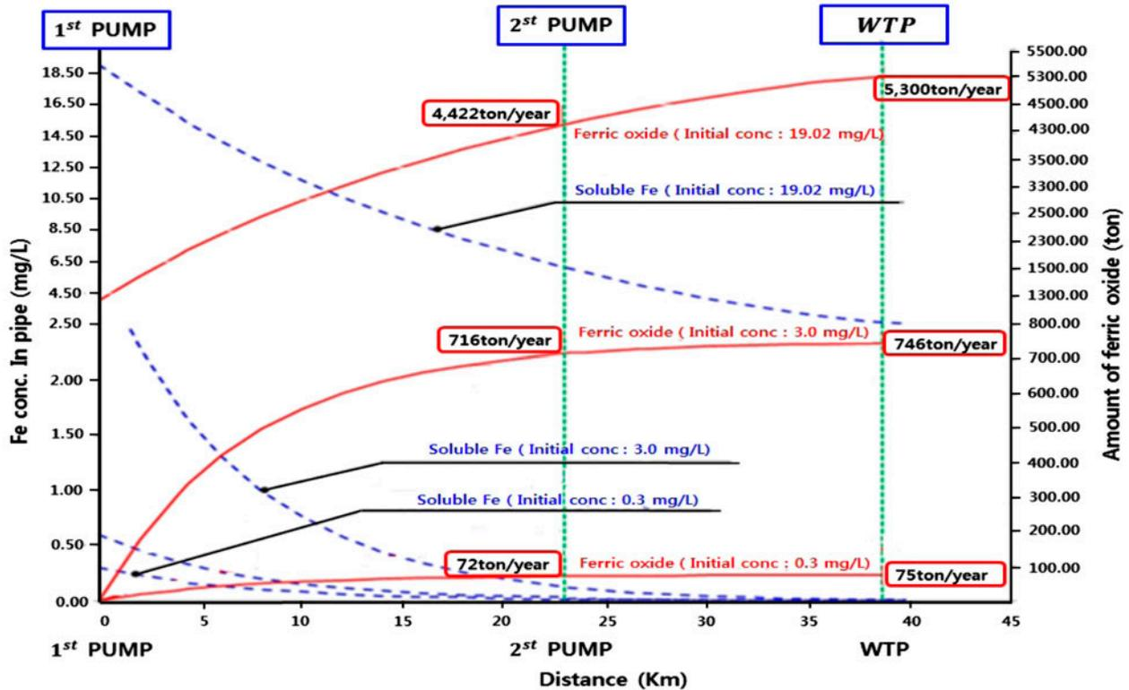
Fig. 6. Product of ferrous oxide depending on different initial soluble Fe.
