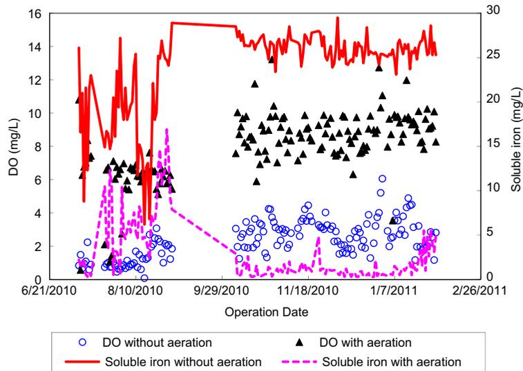
Fig. 5. DO and soluble iron concentrations with and without pretreatment (observed from pilot plant).
