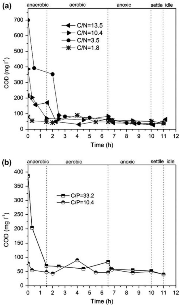
Fig. 6. Effect of different (a) C/N and (b) C/P values on COD removal.
