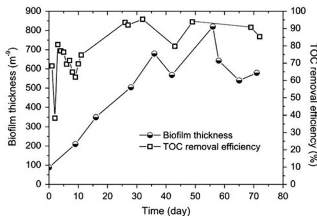
Fig. 2. TOC removal efficiencies and biofilm thicknesses vs. the operation days.
