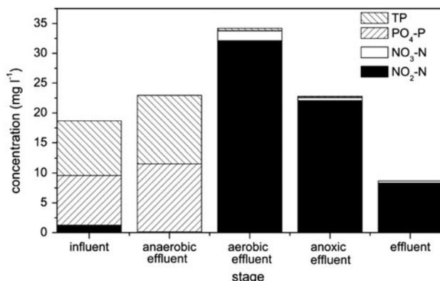
Fig. 8. Effect of  $\text{NO}_3\text{-N}$ ,  $\text{NO}_2\text{-N}$  on the phosphorus removal rate.
