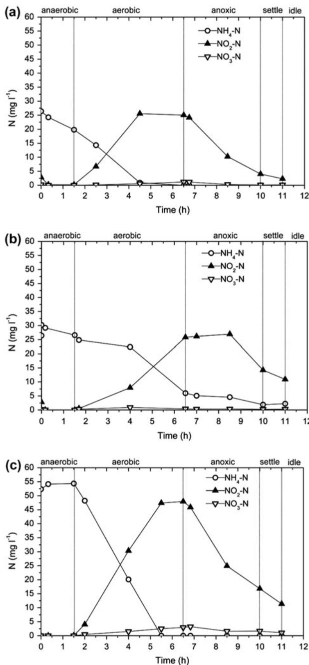
Fig. 7. Effect of the initial  $\text{NH}_4\text{-N}$  on the nitrogen removal rate: (a)  $\text{pH}=7.24$ , temperature from  $19.1$  to  $27.1^\circ\text{C}$ ,  $\text{max}=30.1^\circ\text{C}$ ; (b)  $\text{pH}=7.35$ , temperature from  $21.2$  to  $30.6^\circ\text{C}$ ,  $\text{max}=33.0^\circ\text{C}$ ; and (c)  $\text{pH}=7.34$ , temperature from  $20.7$  to  $30.4^\circ\text{C}$ ,  $\text{max}=33.1^\circ\text{C}$ .
