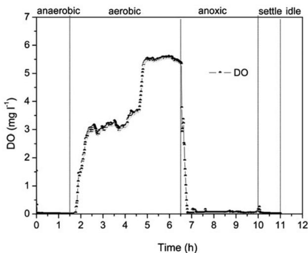
Fig. 4. Oxygen evolution during the SBR process using EFBBR.
