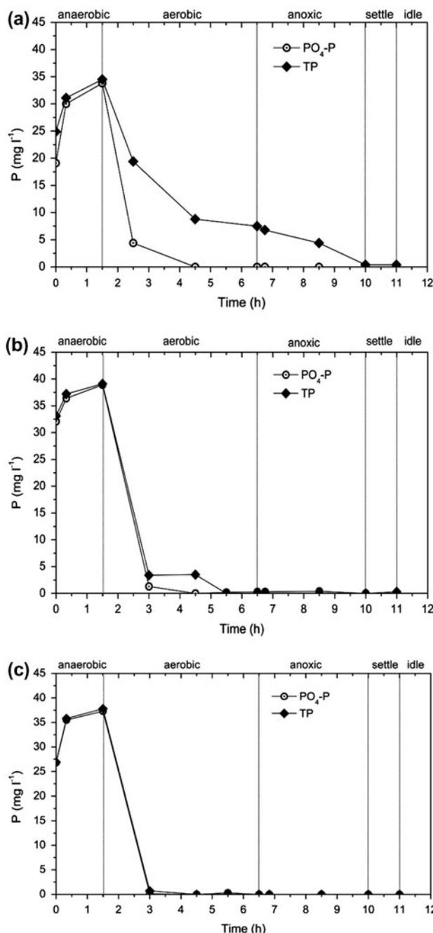
Fig. 9. Effect of temperature on the phosphorus removal (a)  $19.1\text{--}28.4^\circ\text{C}$ ; (b)  $20.4\text{--}23.6^\circ\text{C}$ ; and (c)  $21.9\text{--}23.1^\circ\text{C}$ .
