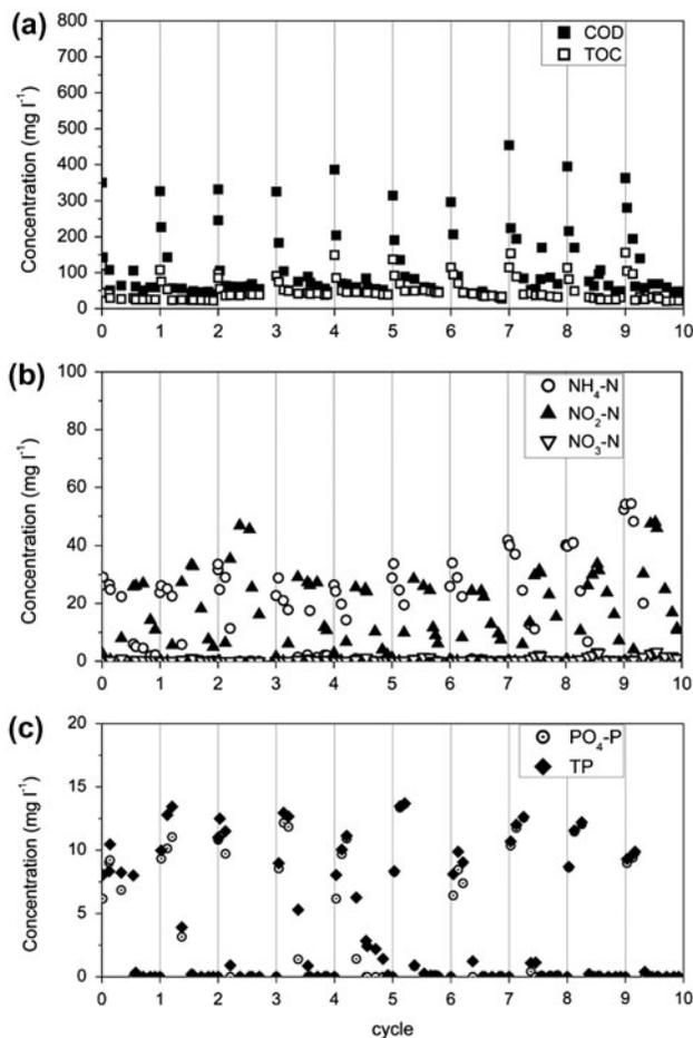
Fig. 5. Nutrient removal using the EFBBR (a) organic removal; (b) nitrogen removal; and (c) phosphorus removal.
