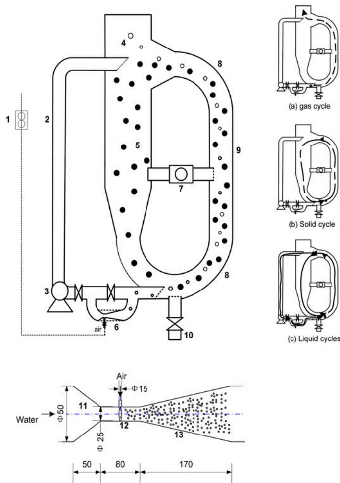
Fig. 1. Schematic diagram of the experimental apparatus.
