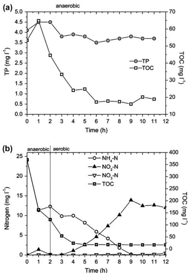
Fig. 3. (a) Phosphorus and (b) Nitrogen concentration changes during anaerobic and/or aerobic period.
