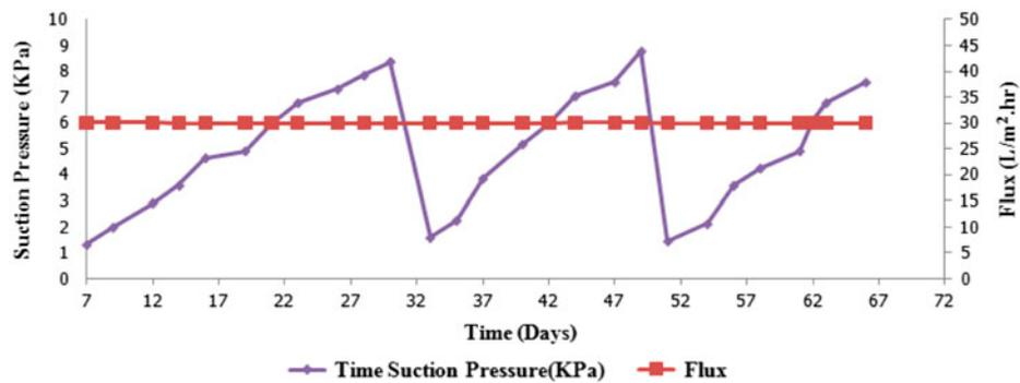
Fig. 10. Transmembrane pressure and membrane permeate flux of the ABR-MBR system.
