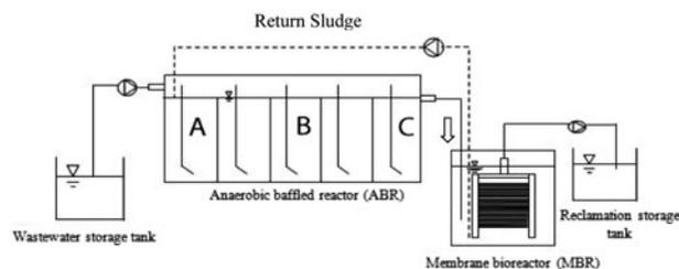
Fig. 1. The schematic diagram of the pilot-scale experimental setup.
