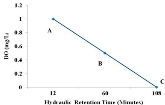
Fig. 6. Oxygen depletion as a function of HRT in the ABR compartment.
