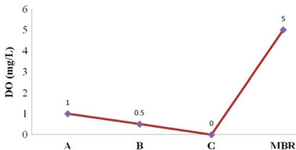
Fig. 2. DO profile in each compartment of the ABR-MBR system.
