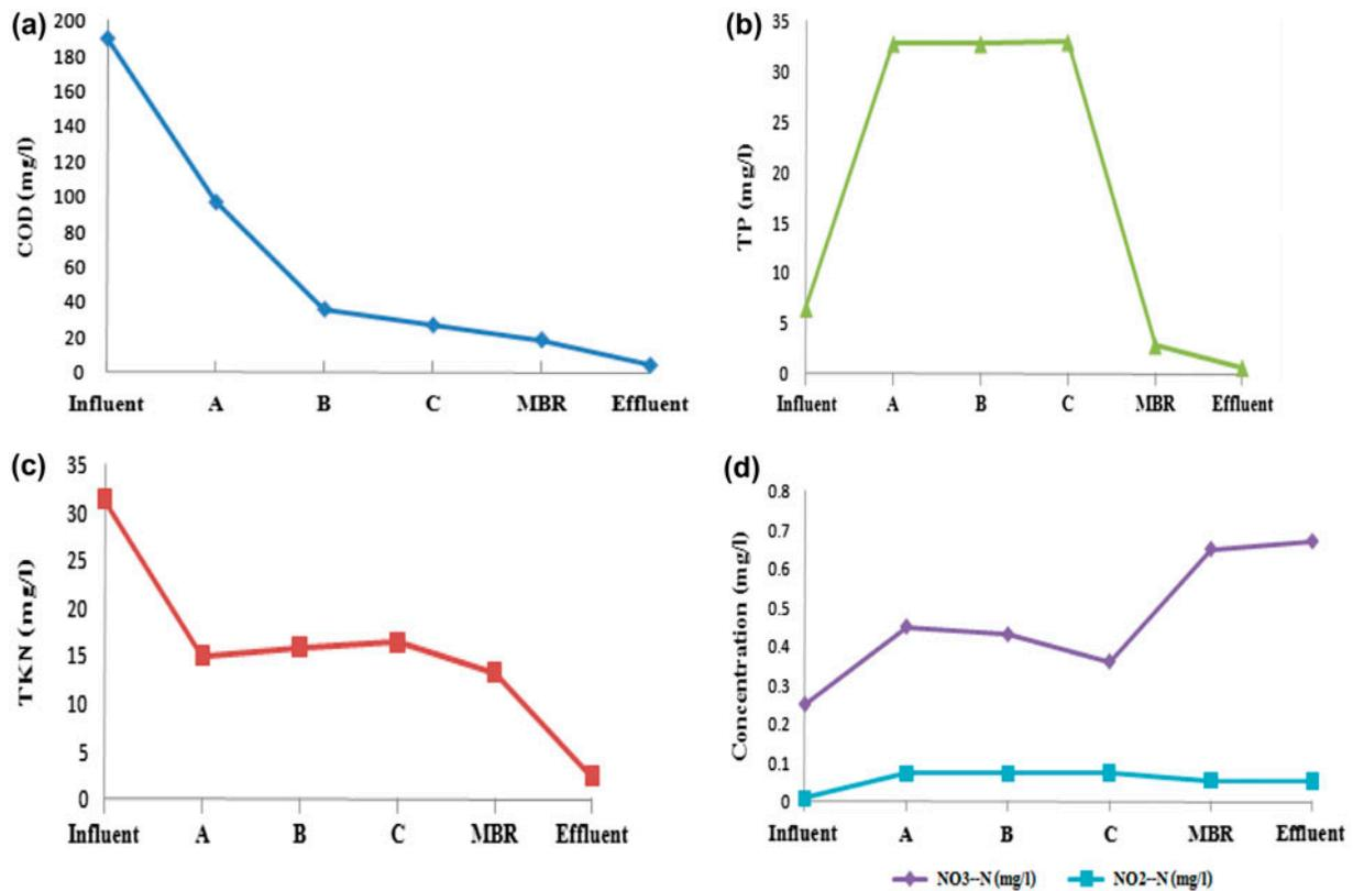
Fig. 8. Profiles of COD (a), TP (b), TKN nitrogen (c), NO<sub>2</sub><sup>-</sup>-N and NO<sub>3</sub><sup>-</sup>-N (d) in each compartment of the ABR-MBR system. Note: A: sample from ABR at A, B: sample from ABR at B, and C: sample from ABR at C; see Fig. 1.
