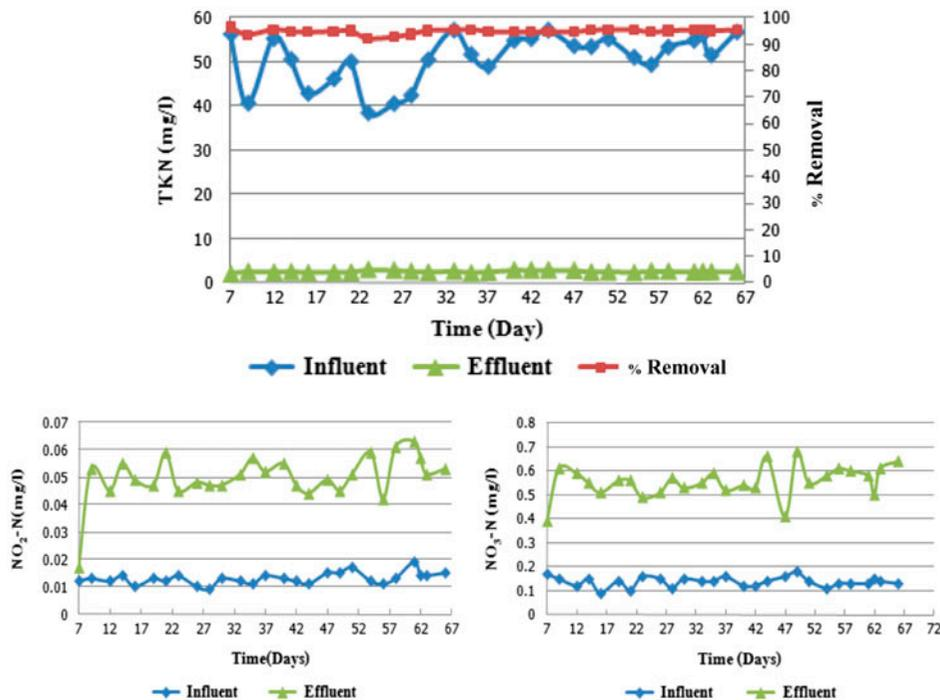
Fig. 4. The variation in TKN-N,  $\text{NO}_2^-$ -N, and  $\text{NO}_3^-$ -N concentrations.
