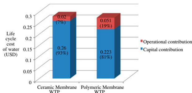
Fig. 3. LCC of produced water from ceramic and polymeric WTPs.
