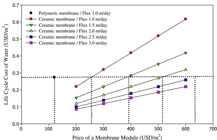
Fig. 4. LCC analysis for different flux and membrane module price.
