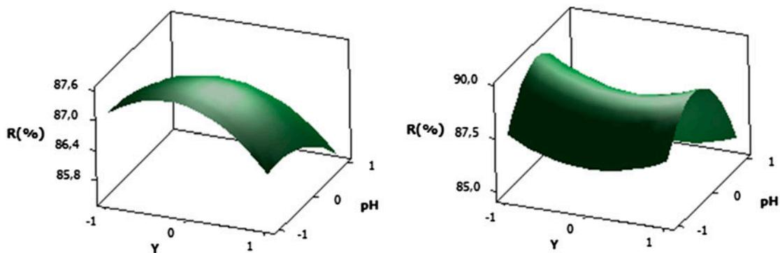
Fig. 8. Response variation— $R$  in the plan:  $Y$ ,  $\text{pH}$ /fixed factor: [dye] = 60 mg/l [BG4 (diagram at left) and BY2 (diagram at right)].
