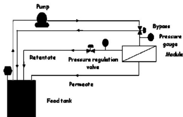
Fig. 1. Schematic representation of the module NF/RO.
