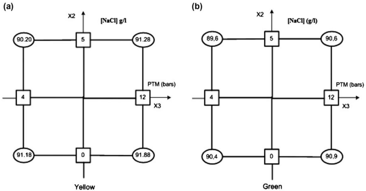
Fig. 6. Interaction between the salt concentration and pressure transmembrane. Retention is marked in ellipses, factors maximum and minimum values in square. (a) For BY2 and (b) for BG4.
