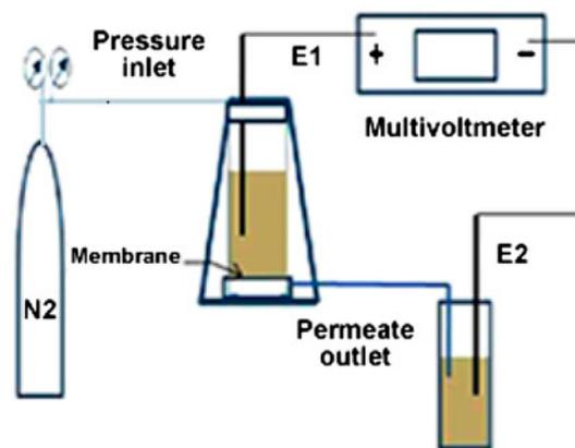
Fig. 2. Schematic representation of the measuring device PE.
