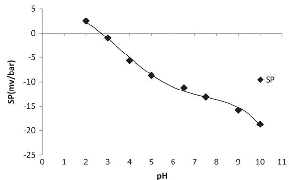
Fig. 3. Behavior of the SP as a function of pH for NF270 (KCl = 10–3 M, T = 20 °C).
