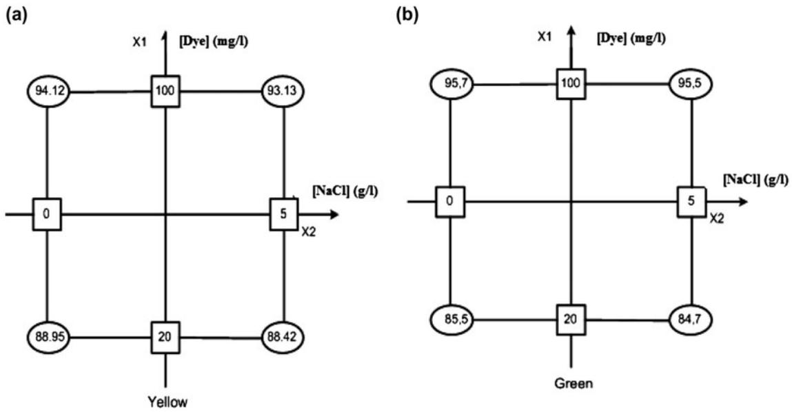
Fig. 5. Interaction between the initial dye concentration and pressure transmembrane. Retention is marked in ellipses, factors maximum and minimum values in square. (a) For BY2 and (b) for BG4.
