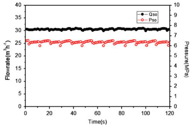
Fig. 9. The flow and pressure curve of the pressurized seawater stream with time.
