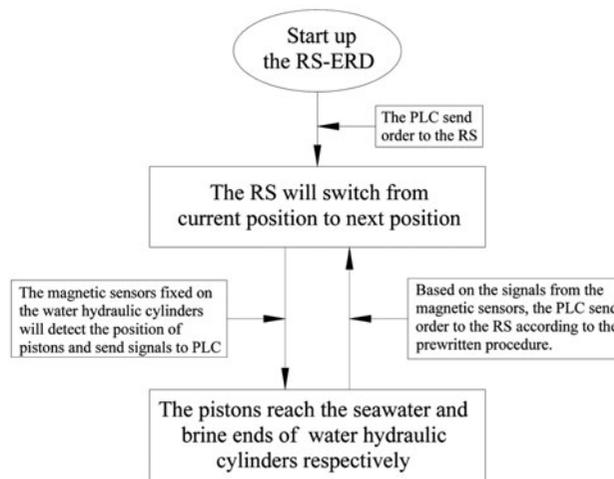
Fig. 2. The control loops for RS-ERD device.
