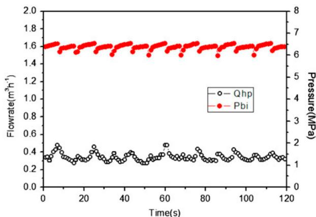
Fig. 10. The flow curve of HP pump with time.
