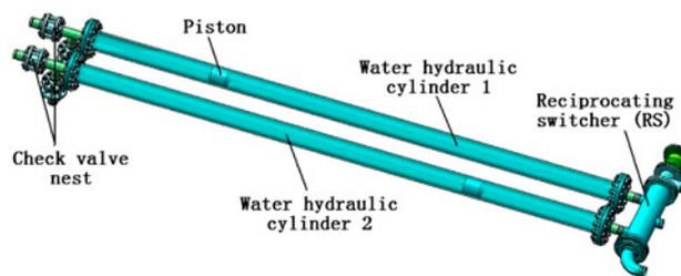
Fig. 1. Basic components of RS-ERD.
