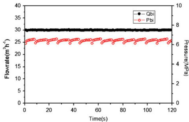
Fig. 8. The flow and pressure curve of the HP brine stream with time.
