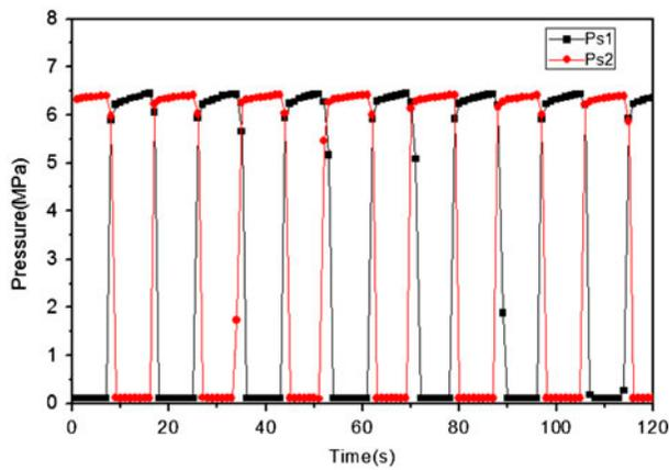
Fig. 7. The pressure curve of the hydraulic cylinder seawater end with time.
