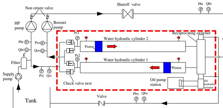
Fig. 5. The flow diagram of RS-ERD test stand.
