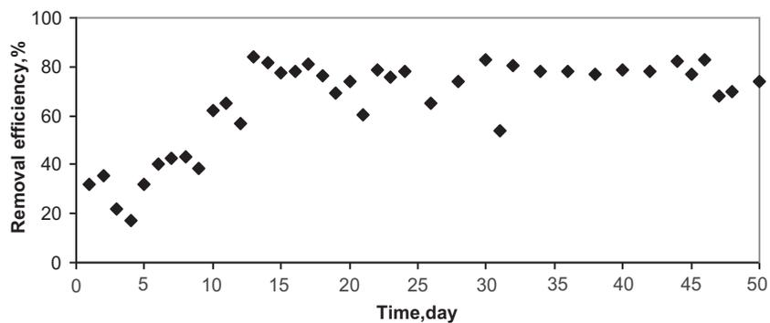
Fig. 7. Removal efficiency of SO<sub>4</sub><sup>2-</sup>.
