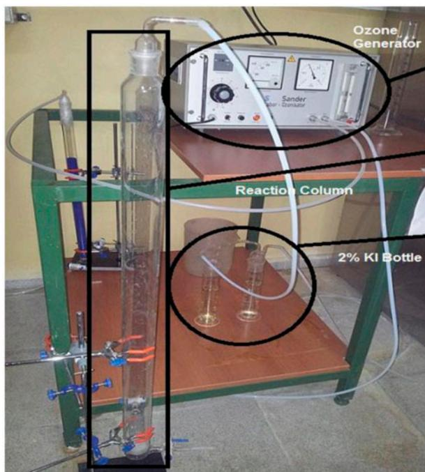
Fig. 1. Photograph of the ozone setup.
