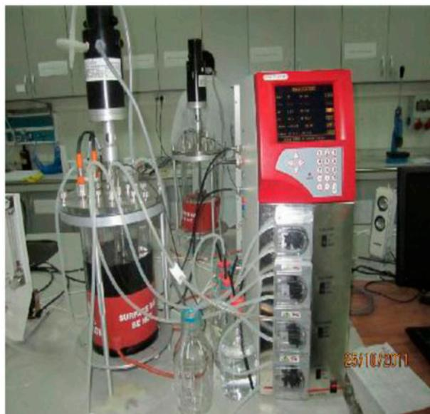
Fig. 2. Photograph of the anaerobic fermenter.
