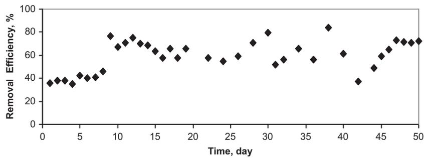
Fig. 5. Removal efficiency of DCOD.
