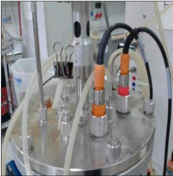
Fig. 3. Photograph of pH, ORP, and temperature probes connected to the fermentor system.
