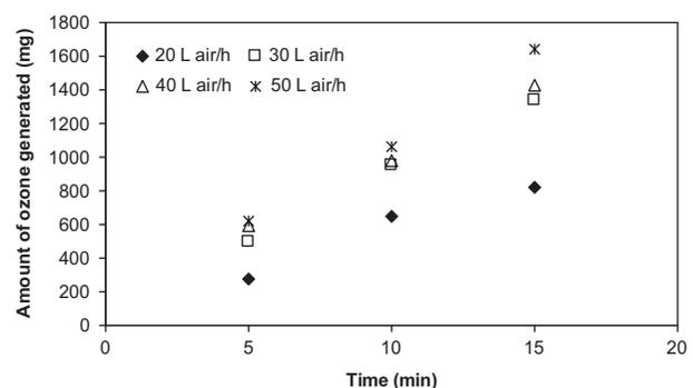
Fig. 4. The amount of ozone generated at different ozone dose and reaction time (volume of wastewater sample = 500 mL).
