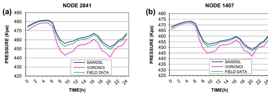
Fig. 11. Observed vs. simulated pressure values in both SAWDSL and Voronoi methods (a) in node 2841 at M. Kanari str.; and (b) in node 235 at M. Psaron str.
