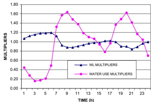
Fig. 9. Real losses and the rest water consumption daily patterns applied to the model.
