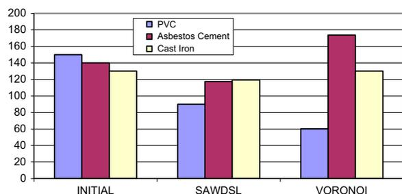
Fig. 14. Initial and modified (through model calibration) values of Haazen Williams C factor of the main three WDN’s materials.
