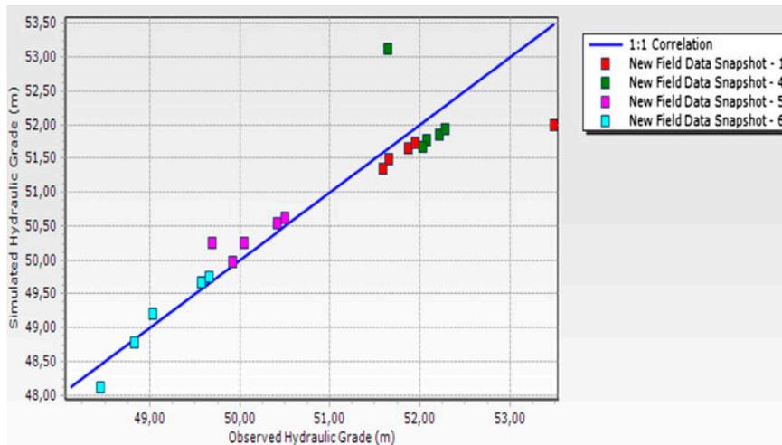
Fig. 12. Correlation between observed and simulated HG in SAWDSL method.
