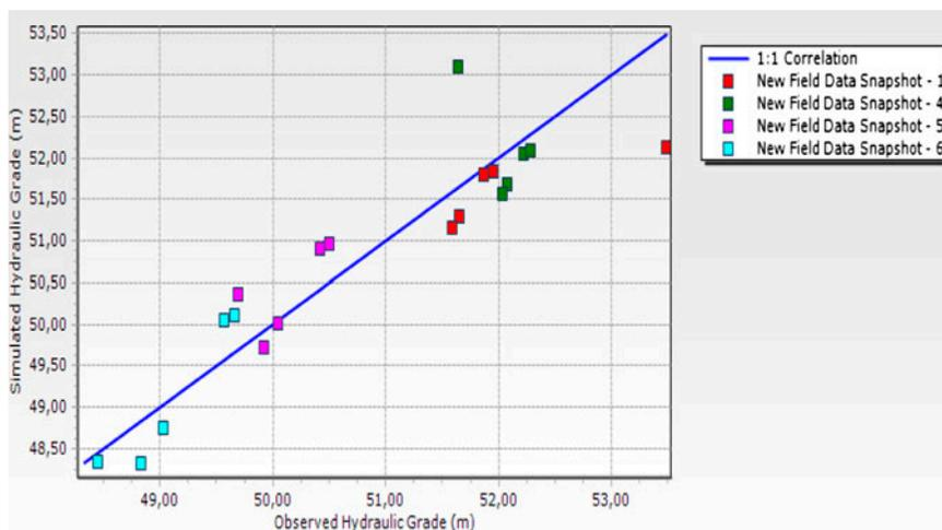
Fig. 13. Correlation between observed and simulated HG in Voronoi method.
