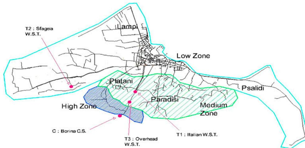
Fig. 4. Pressure zones, water storage tanks in Kos Town water network.
