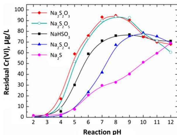
Fig. 4. Influence of reaction pH on Cr(VI) removal (Initial Cr(VI) = 100 µg/L,  $C_{\text{ISR}} = 10$  mg S/L, reaction time 24 h, and reaction temperature  $20 \pm 1^\circ\text{C}$ ).
