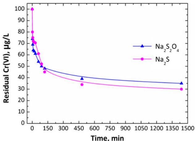
Fig. 7. Reaction kinetics of  $\text{Cr(VI)}$  (Initial  $\text{Cr(VI)} = 100 \mu\text{g/L}$ ,  $\text{C}_{\text{ISR}} = 20 \text{ mg S/L}$ , and pH 7).
