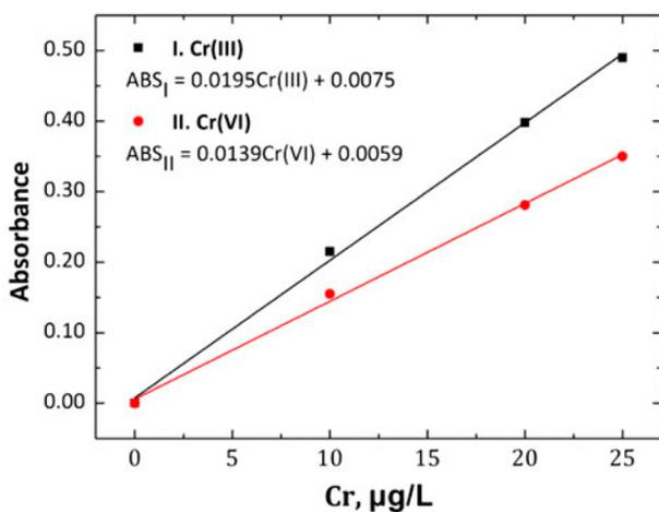
Fig. 2. Calibration curves for I: Cr(III) and II: Cr(VI) using the GFAAS.
