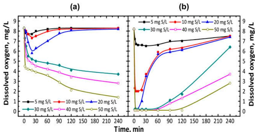
Fig. 6. Dissolved oxygen concentration as a function of reaction time and  $\text{Na}_2\text{S}$  (a) and  $\text{Na}_2\text{S}_2\text{O}_4$  (b) dose. (Initial  $\text{Cr(VI)} = 100 \mu\text{g/L}$ , pH 7).
