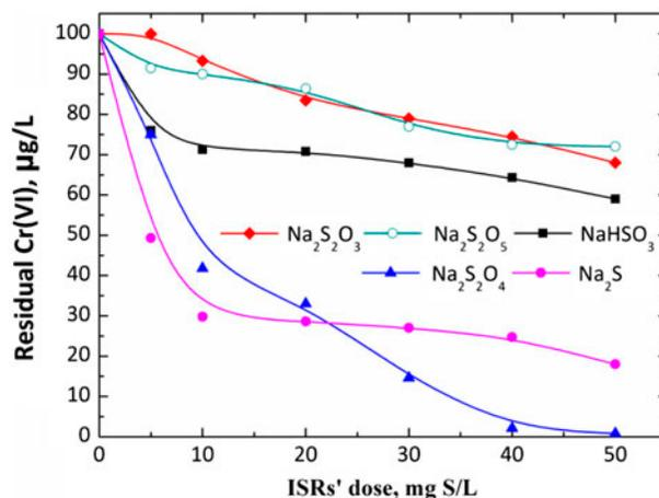
Fig. 5. Influence of ISRs dose on residual Cr(VI) concentration. (Initial Cr(VI) = 100 µg/L, pH 7, reaction time 24 h, and reaction temperature  $20 \pm 1^\circ\text{C}$ ).
