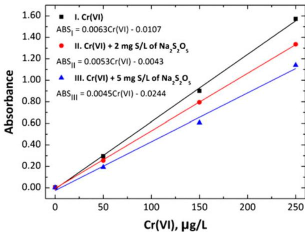
Fig. 1. Absorbance as a function of Cr(VI) concentration using the 1,5-diphenylcarbazide method. I: Cr(VI), II: Cr(VI) with 2 mg S/L of  $\text{Na}_2\text{S}_2\text{O}_5$  added, and III: Cr(VI) with 5 mg S/L of  $\text{Na}_2\text{S}_2\text{O}_5$  added.
