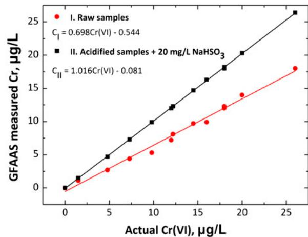
Fig. 3. Cr(VI) in natural water matrix determined by GFAAS against Cr(III) calibration curve. I: Raw samples and II: Acidified samples with 20 mg/L  $\text{NaHSO}_3$  added.
