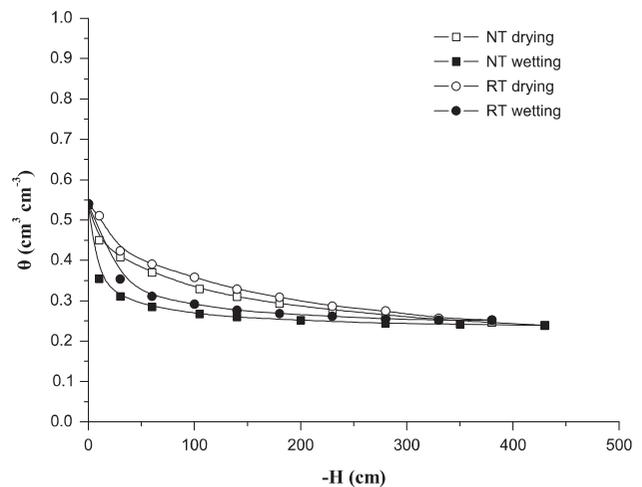
Fig. 2. Experimental water retention curves during drying and wetting for the NT and RT bare soils.
