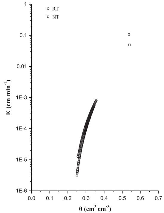
Fig. 4. Hydraulic conductivity as a function of water content for the NT and RT bare soils obtained by outflow data using the Valiantzas et al. equation (Eq. (3)) and water retention data.
