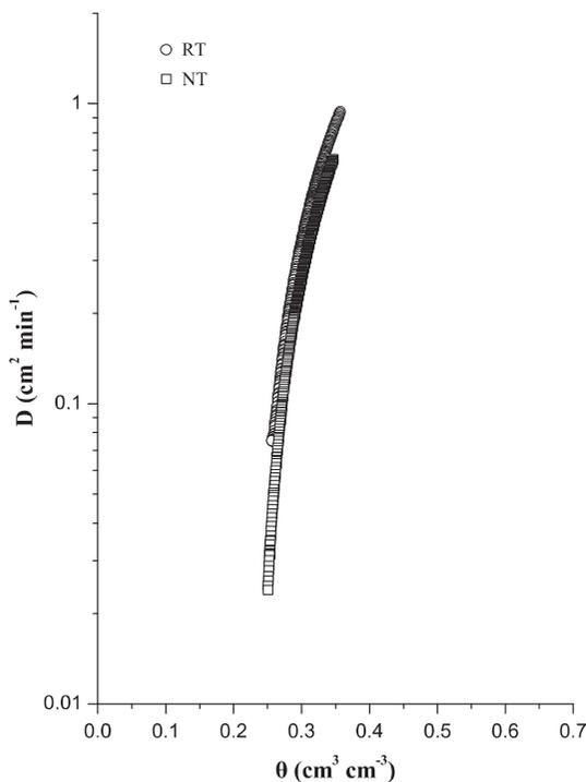
Fig. 3. Soil diffusivity as a function of water content for the NT and RT bare soils.
