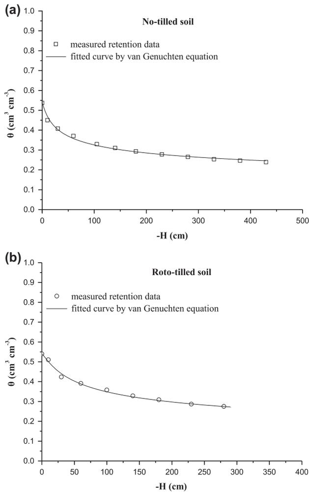
Fig. 5. Experimental and fitted (using the van Genuchten equation) water retention curves during drying for the NT (a) and RT (b) bare soils.
