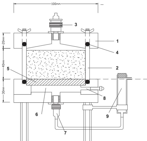
Fig. 1. Richards' pressure cell: (1) plexiglass plate, (2) cylinder, (3) connecting valve, (4) elastic O-rings, (5) porous plate, (6) water reservoir, (7) water exit, (8) air exit, and (9) water reservoir.
