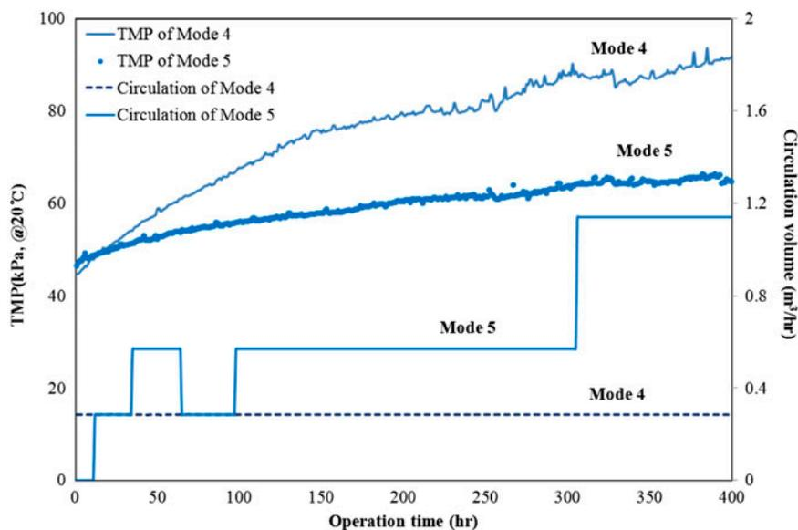
Fig. 7. Effect of linear velocity variation on TMP.
