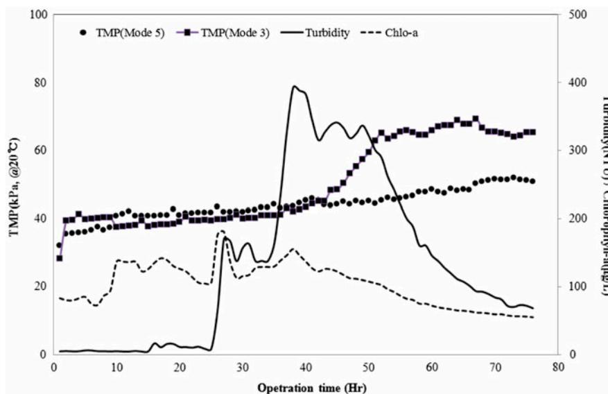
Fig. 6. Comparison of TMP between dead-end and cross-flow modes.
