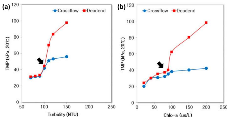
Fig. 3. Decision of operation mode based on the raw water characteristics. (a) Effect of turbidity on TMP. (b) Effect of algae on TMP.
