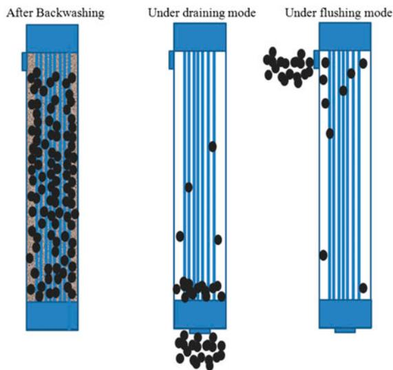
Fig. 9. Discharging suspended solids between draining and flushing.
