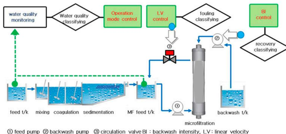
Fig. 1. The detailed process of hybrid MF pilot system.
