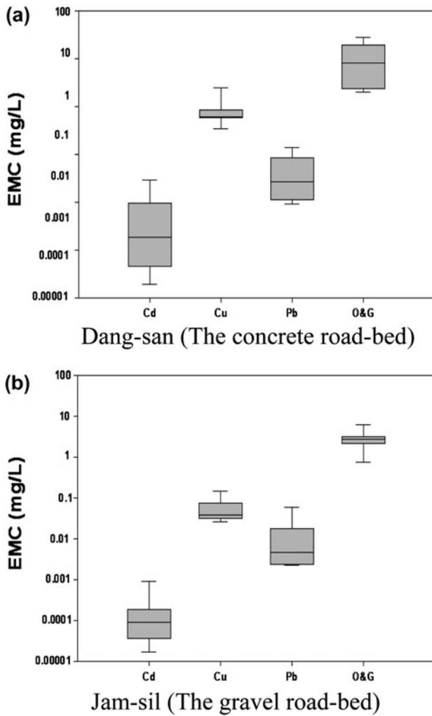
Fig. 4. Analysis of heavy metal and O&G EMC: (a) Dang-san (the concrete road-bed) and (b) Jam-sil (the gravel road-bed).
