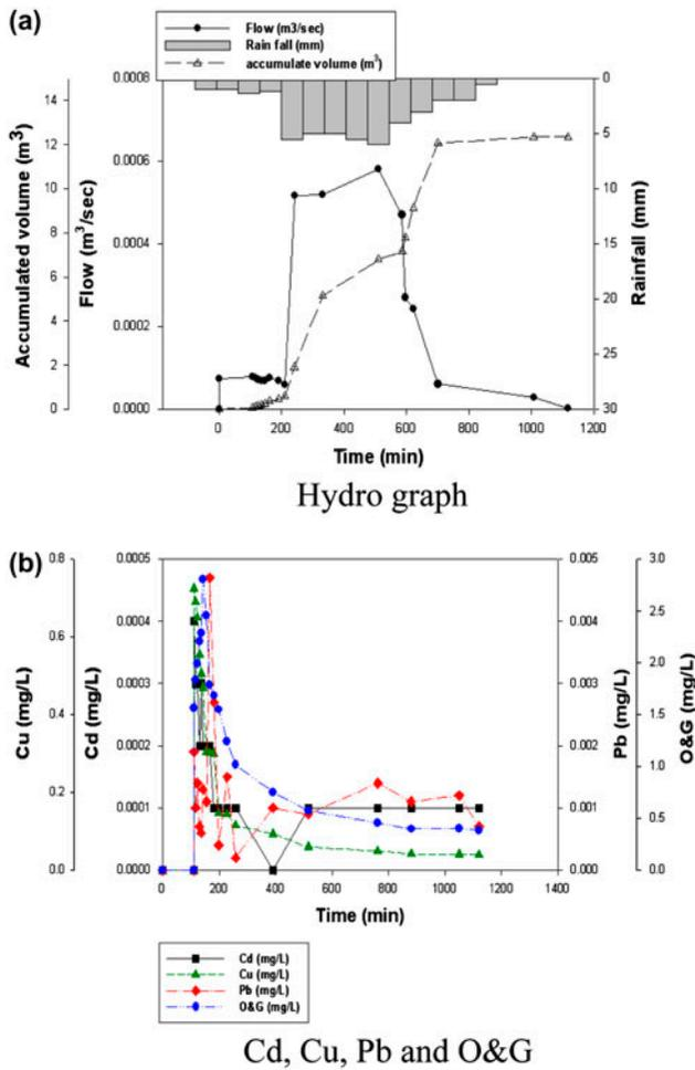
Fig. 2. Hydro-polluto graph of concrete road-bed area: (a) Hydro graph and (b) Cd, Cu, Pb, and O&G.
