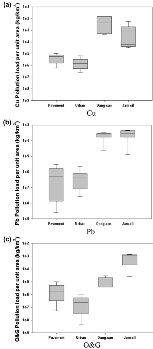
Fig. 5. Analysis of the pollutant load per unit area: (a) Cu, (b) Pb, and (c) O&G.
