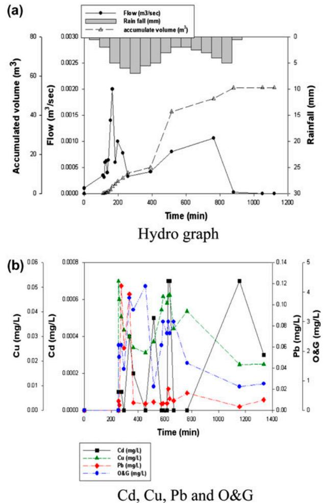
Fig. 3. Hydro-polluto graph of gravel road-bed area: (a) Hydro graph and (b) Cd, Cu, Pb, and O&G.
