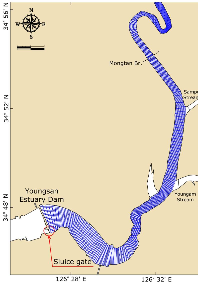
Fig. 3. Horizontal grid developed for the Youngsan River for this study (only downstream areas are shown in this figure).
