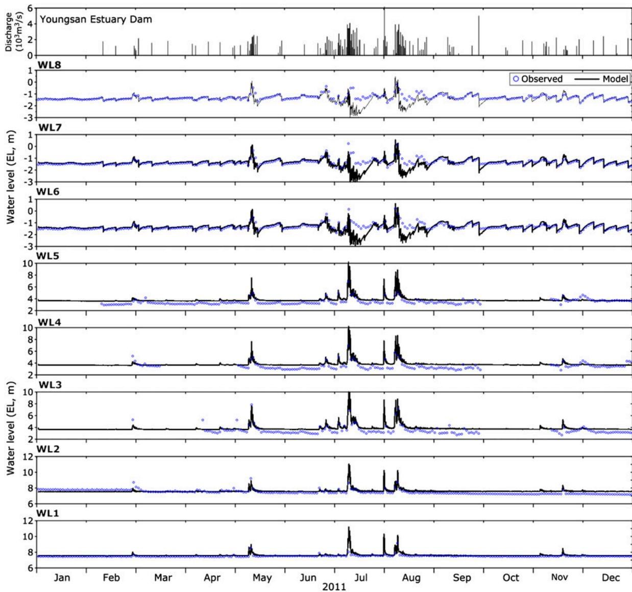
Fig. 5. Water level calibration results in selected locations (Fig. 1) of the Youngsan River.
