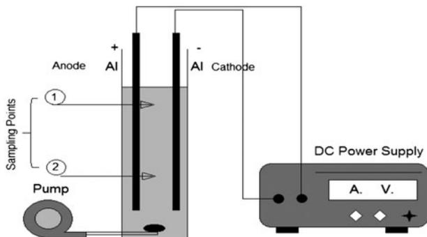
Fig. 2. Schematic figure of decolorization unit.
