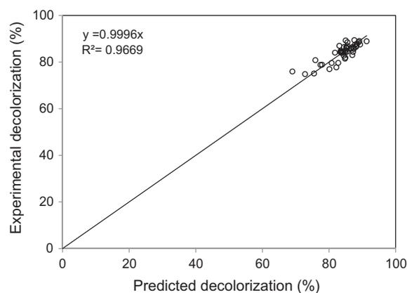
Fig. 4. Predicated value vs. actual value for the decolorization efficiency.
