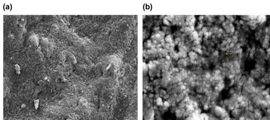
Fig. 6. SEM of the electrocoagulation sludge, 10  $\mu\text{m}$  (a) and 1  $\mu\text{m}$  (b).
