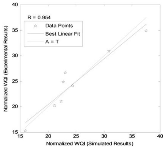
Fig. 4. Regression plot on WQI (experimental vs. predicted) using the CCME Method with five input variables, 10 processing elements in the hidden layer, and one output variable.
