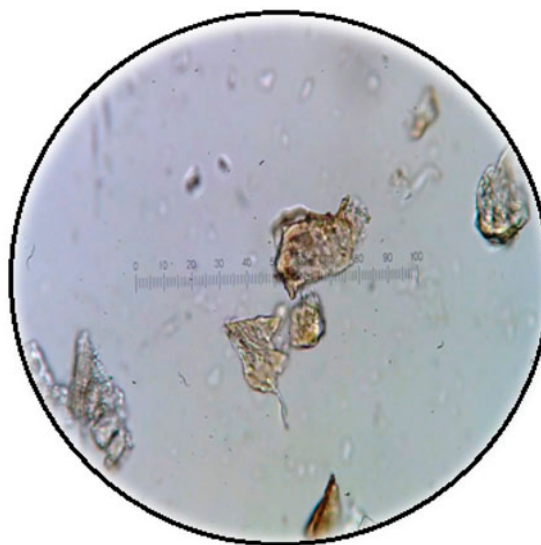
Fig. 4. Binocular micrograph of RHA (magnification: \times 40 ).
