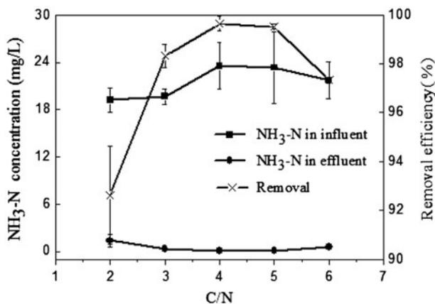
Fig. 3. AN removal performance of ICMBR under different C/N ratio.
