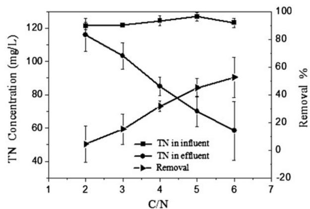
Fig. 4. TN removal performance of ICMBR under different C/N ratio.
