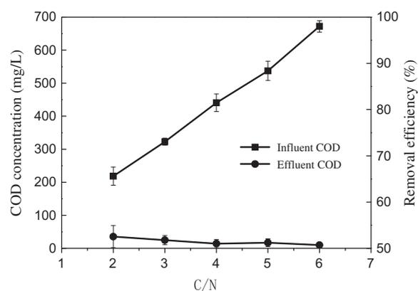
Fig. 2. COD removal performance of ICMBR under different C/N ratio.
