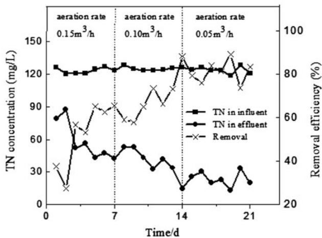
Fig. 7. TN removal performance of ICMBR under different aeration ratio.
