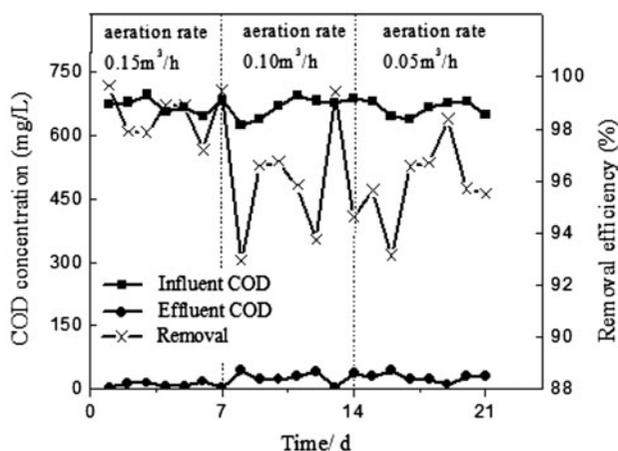
Fig. 5. COD removal performance of ICMBR under different aeration ratio.
