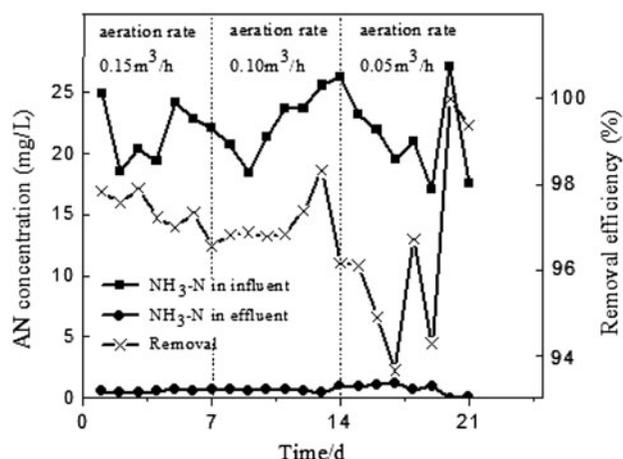
Fig. 6. AN removal performance of ICMBR under different aeration ratio.
