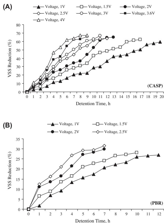
Fig. 3. The percentage of VSS reduction under applied currents of electrochemical process (A) Biowaste from CASP, (B) Biowaste from PBR.
