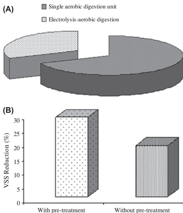
Fig. 6. Comparative evaluation on the necessity of electrolysis process as a preconditioning step of aerobic digestion (A) Overall footprint area requirement, (B) VSS reduction under aerobic condition at 3 d detention time.
