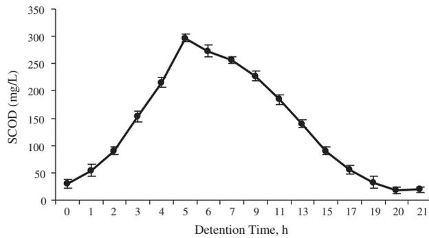
Fig. 4. The profile of soluble COD concentration at different detention time under applied voltage power of 2 V.
