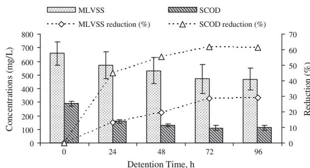
Fig. 5. The variation of VSS and SCOD concentrations during the aerobic digestion of electrolyzed sludge.
