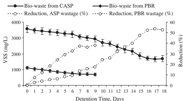
Fig. 2. The compression of VSS reduction under aerobic condition.
