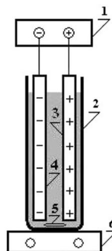
Fig. 1. Schematic appearance of bench scale electrochemical process (1—DC power supply, 2—electrolysis cell, 3—cathode, 4—anode, 5—bar stirrer, and 6—magnetic stirrer).
