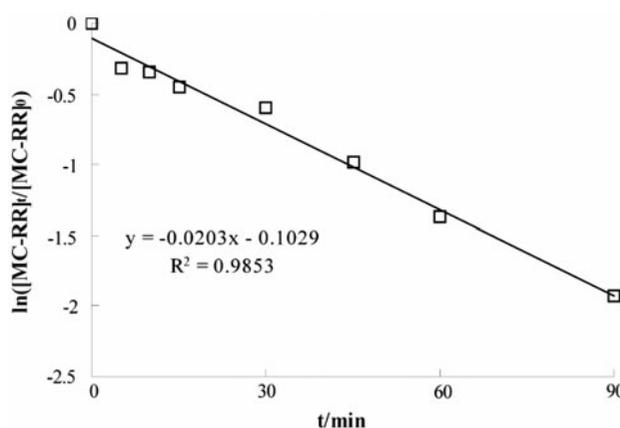
Fig. 4. Pseudo-first-order kinetic plot of MC-RR oxidation reaction (pH:  $7.0 \pm 0.1$ ; MC-RR initial concentration:  $461.5 \mu\text{g/L}$ ;  $\text{O}_3$  concentration:  $0.82 \mu\text{g/L}$ ).
