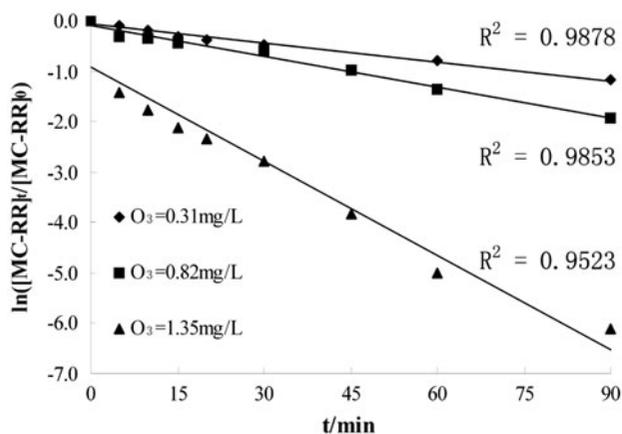
Fig. 5. Effect of the initial  $O_3$  dose on the MC-RR degradation (pH:  $7.0 \pm 0.1$ ; MC-RR initial concentration:  $461.5 \mu\text{g/L}$ ;  $O_3$  concentrations:  $0.31$ ,  $0.82$  and  $1.35 \text{ mg/L}$ ).
