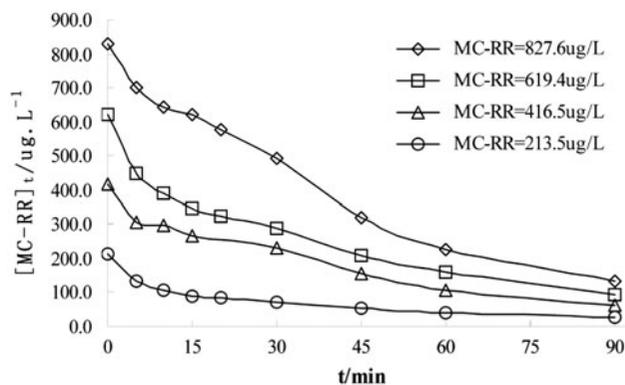
Fig. 6. Variation of residual of MC-RR with reaction time under different initial concentrations (pH:  $7.0 \pm 0.1$ ;  $O_3$  concentration:  $0.82 \text{ mg/L}$ ; MC-RR initial concentrations:  $213.5$ ,  $416.5$ ,  $619.4$ , and  $827.6 \mu\text{g/L}$ ).
