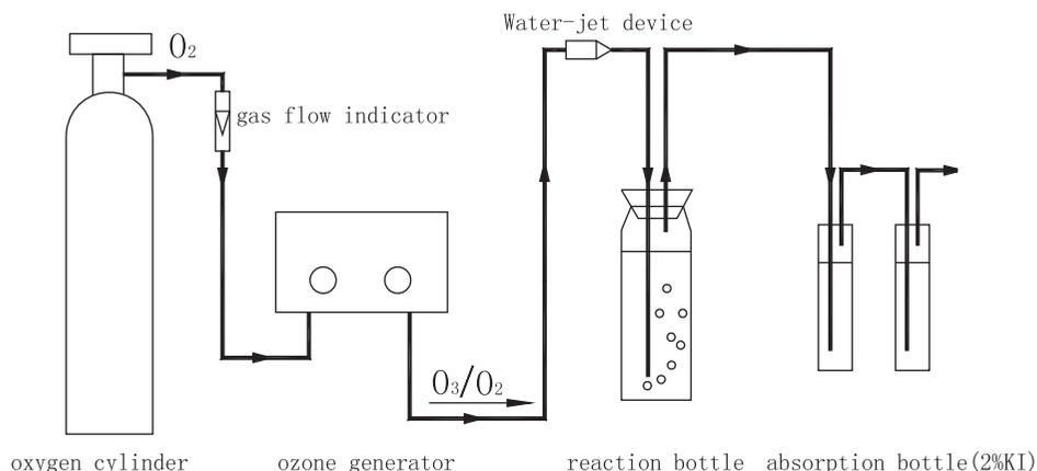
Fig. 1. Schematic diagram of the ozonation system.
