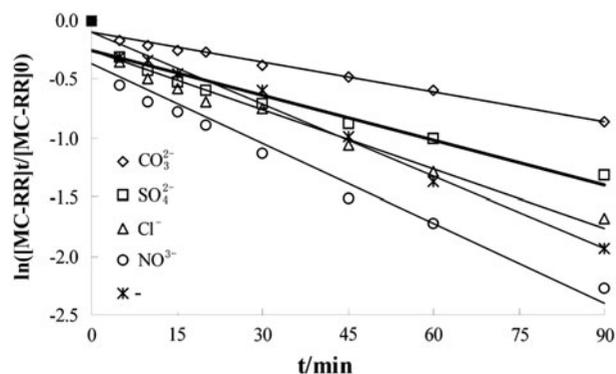
Fig. 8. Effects of anions on the degradation of MC-RR by Ozonation (pH:  $7.0 \pm 0.1$ ; MC-RR initial concentration: 416.5  $\mu\text{g/L}$ ;  $\text{O}_3$  concentration: 0.82 mg/L; the concentrations of  $\text{CO}_3^{2-}$ ,  $\text{SO}_4^{2-}$ ,  $\text{Cl}^-$  and  $\text{NO}_3^-$ : 10 mmol/L).
