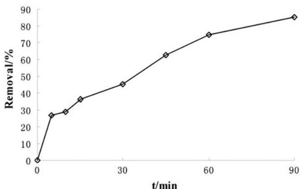
Fig. 3. MC-RR removal by ozonation vs. reaction time (pH:  $7.0 \pm 0.1$ ; MC-RR initial concentration:  $461.5 \mu\text{g/L}$ ;  $\text{O}_3$  concentration:  $0.82 \text{ mg/L}$ ).
