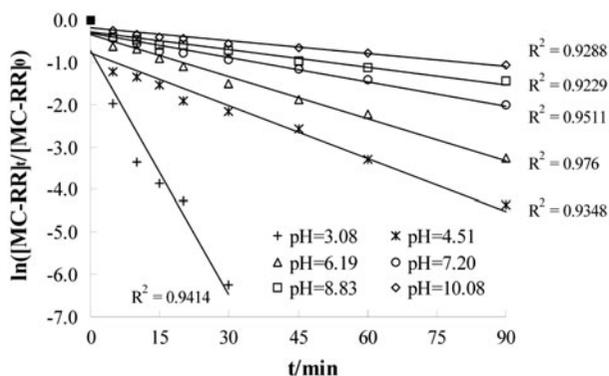
Fig. 7. Effect of solution pH on the MC-RR ozonation (MC-RR initial concentration: 416.5  $\mu\text{g/L}$ ;  $\text{O}_3$  concentration: 0.82 mg/L; pH: 3.08, 4.51, 6.19, 7.20, 8.83, and 10.08).
