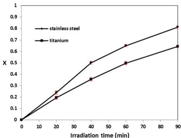
Fig. 8. The effect of anode material on decolorization efficiency in EAP process,  $\text{pH} = 5.4$ ,  $\Delta V = 4 \text{ V}$ ,  $c_0 = 15 \text{ mg L}^{-1}$ ,  $I = 16 \text{ W m}^{-2}$ .
