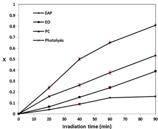
Fig. 5. The promoting effect of electrical field on the decolorization efficiency,  $\text{pH} = 5.4$ ,  $\Delta V = 4 \text{ V}$ ,  $c_0 = 15 \text{ mg L}^{-1}$ ,  $I = 16 \text{ W m}^{-2}$ .
