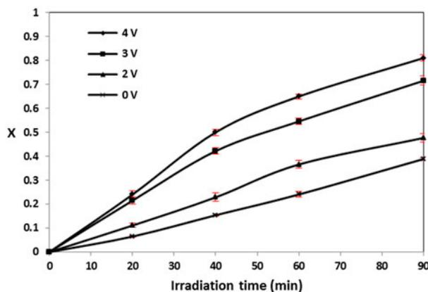
Fig. 7. Effect of potential difference on the decolorization efficiency in EAP process with ZnO/Stainless steel anode and stainless steel cathode,  $\text{pH} = 5.4$ ,  $c_0 = 15 \text{ mg L}^{-1}$ ,  $I = 16 \text{ W m}^{-2}$ .
