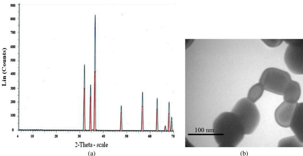
Fig. 3. Characteristics of the used ZnO nanoparticles: (a) XRD pattern (b) TEM image. The red lines show standard ZnO peaks.
