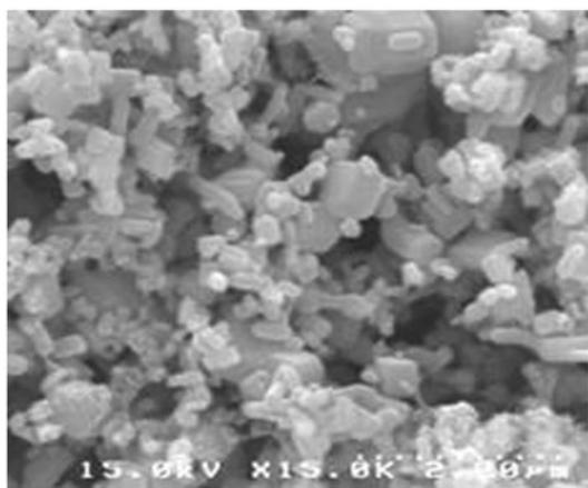
Fig. 4. SEM image of stainless steel surface after the immobilization of ZnO nanoparticles.
