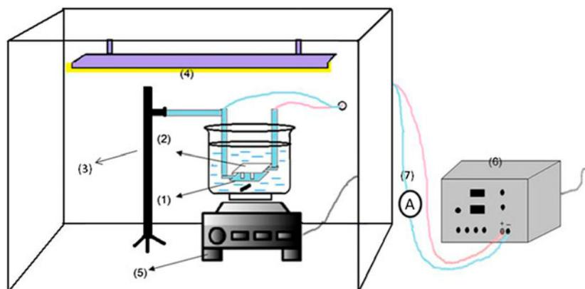
Fig. 1. Scheme of EAP setup, (1) Stainless steel cathode, (2) ZnO/Stainless steel or ZnO/titanium anode, (3) Support, (4) UV lamp, (5) Magnetic stirrer, (6) DC supply, (7) Ampere meter.
