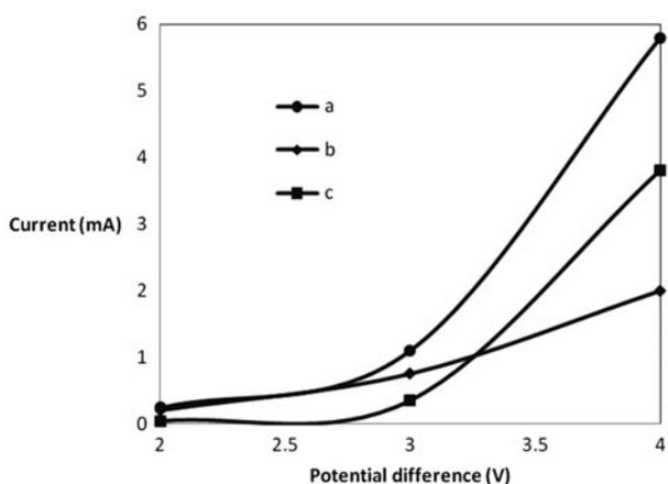
Fig. 6. “Potential difference vs. current” curves for a system containing ZnO/Stainless steel anode and stainless steel cathode in Reactive Navy Blue SP-BR solution,  $\text{pH} = 5.4$ ,  $c_0 = 15 \text{ mg L}^{-1}$ , under (a): UV irradiation ( $I = 16 \text{ W m}^{-2}$ ) (b): darkness. Curve “c” shows the difference of curves “a” and “b”.
