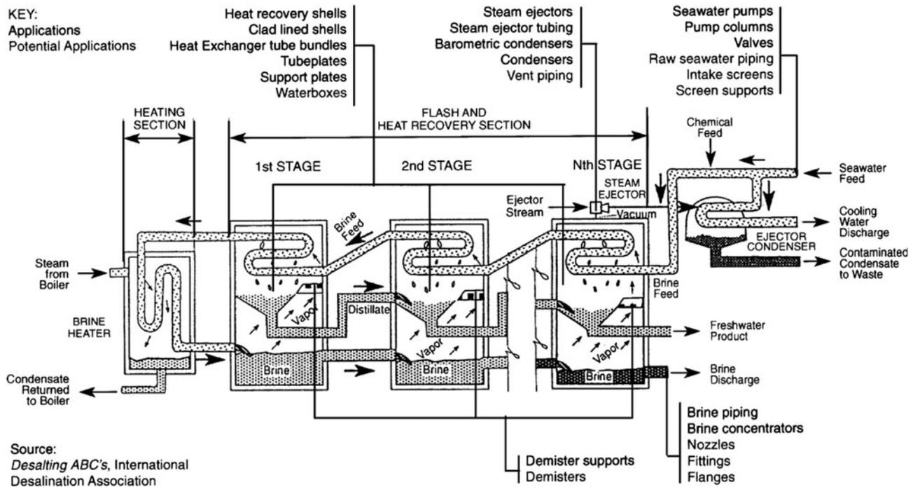
Fig. 1. Diagram of a MSF distillation plant.
