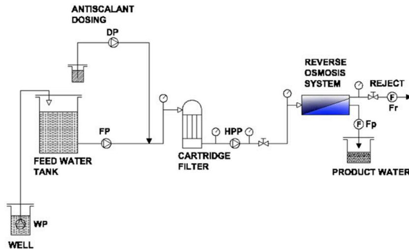
Fig. 1. Desalination plant diagram, where WP, well pump; FP, feed pump; DP, dosing pump; HPP, high pressure pump; F, flowmeter; Fr, rejection flow; Fp, product flow.
