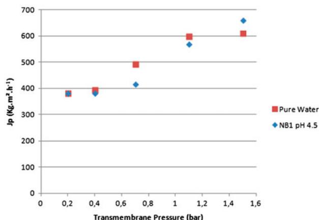
Fig. 7. Behavior of permeation fluxes at each pressure during the MF in total recirculation mode.
