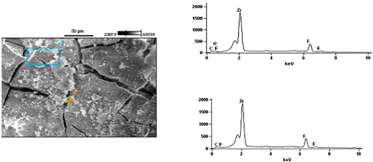
(b) SEM-EDS Cationic Membrane – HDX100 – Central Compartment
