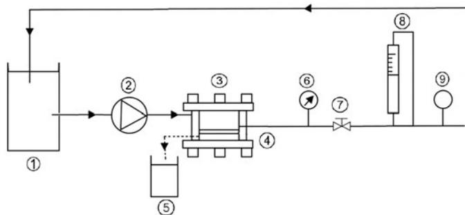
Fig. 4. Setup of the permeation module. 1—Feed tank, 2—Pump, 3—Permeation cell, 4—Membrane, 5—Permeate sample, 6—Manometer, 7—Pressure regulation valve, 8—Rotameter, and 9—Thermometer.
