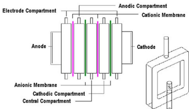
Fig. 2. Schematic ED bench cell with all compartments and the ionic exchange membranes alternately arranged being represented.
