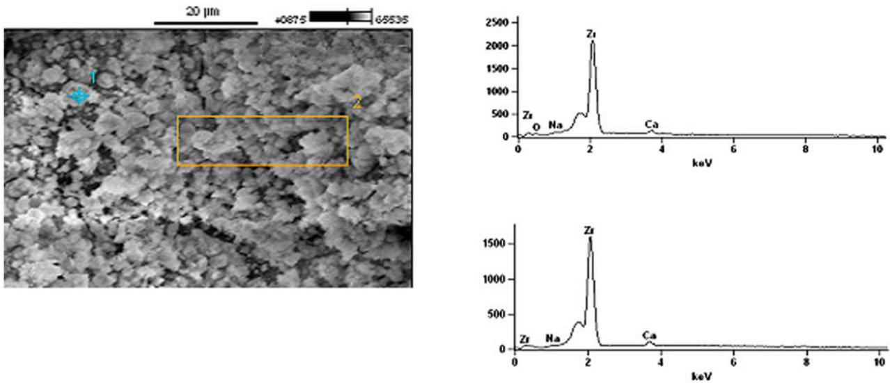
(a) SEM-EDS Anionic Membrane – HDX200 – Central Compartment
