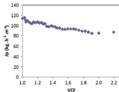
Fig. 9. Behavior of permeation flux in NF with controlled pH 10, in concentration mode.
