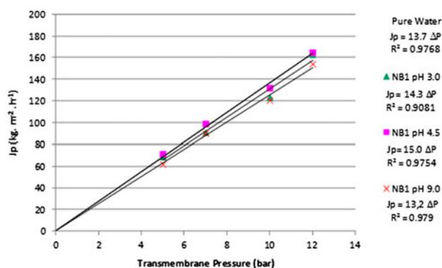
Fig. 8. Behavior of NB1 at different pH values in NF in total recirculation mode.
