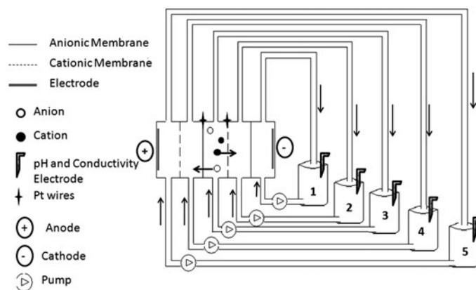
Fig. 3. Setup of the ED module. 1—Electrode compartment (cathode), 2—Cathodic compartment, 3—Central compartment, 4—Anodic compartment, and 5—Electrode compartment (anode).
