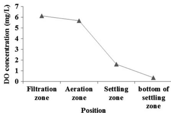
Fig. 7. DO concentration at different zones of the reactor.
