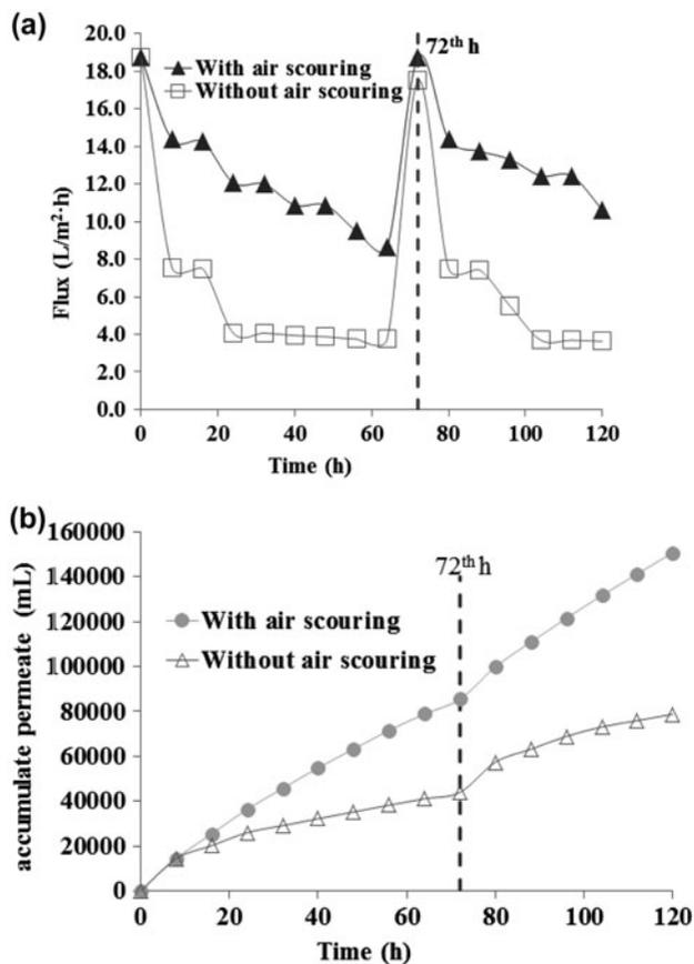
Fig. 5. Effect of air scouring of membrane on the (a) permeate flux and (b) cumulative permeate volume.
