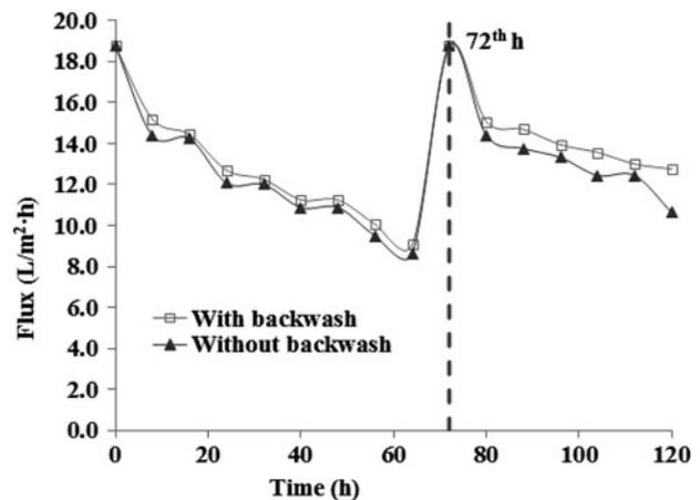
Fig. 6. Effect of backwash on the permeate flux.
