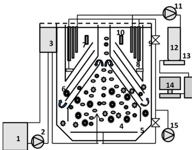
Fig. 2. MBR with inclined plate: (1) feed tank; (2) influent pump; (3) constant head tank; (4) aeration zone; (5) air diffuser; (6) settling zone; (7) filtration zone; (8) air diffuser; (9) membranes; (10) baffles; (11) effluent pump; (12) permeate tank; (13) balance scale; (14) data recorder; and (15) air pump.
