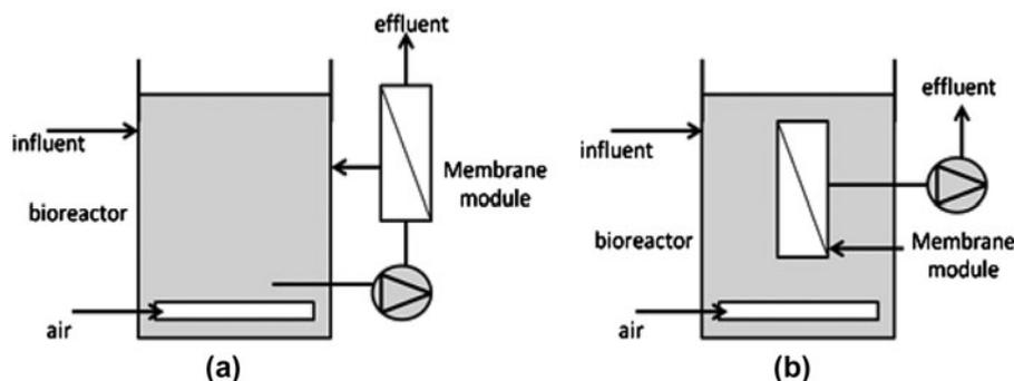
Fig. 1. Schematic diagrams of basic MBR configuration. (a) Side sMBR with membrane module and (b) iMBR with membrane module immersed in the bioreactor.
