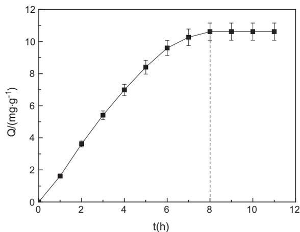
Fig. 4. Kinetic adsorption curve. Temperature: 25°C; pH = 6; initial concentration of TNT: 100 mg L<sup>-1</sup>.
