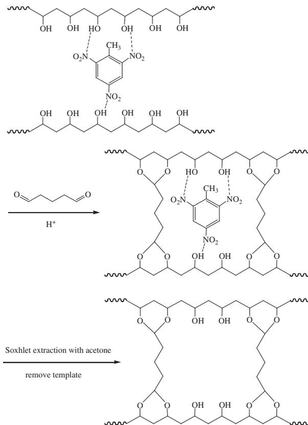
Fig. 1. Preparation scheme of MIP-CPVA.
