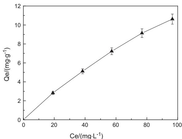
Fig. 5. Adsorption isotherm of MIP-CPVA towards TNT. Temperature: 25°C; pH = 6; Adsorption time: 8 h.
