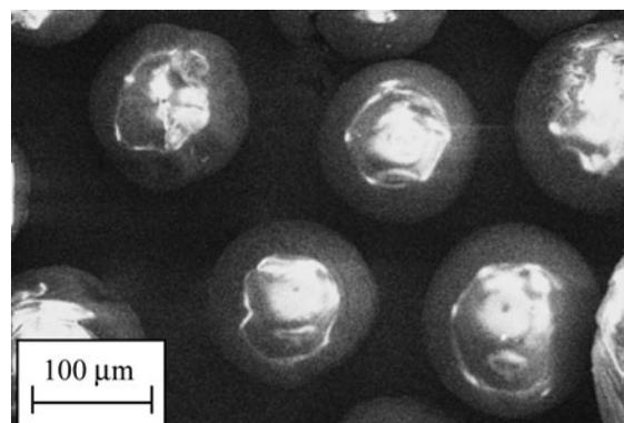
Fig. 3. SEM image of MIP-CPVA microspheres.
