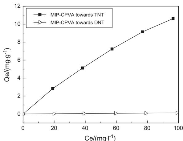
Fig. 7. Adsorption isotherms of MIP-CPVA towards DNT and TNT. Temperature: 25°C; pH=6; Adsorption time: 8 h.
