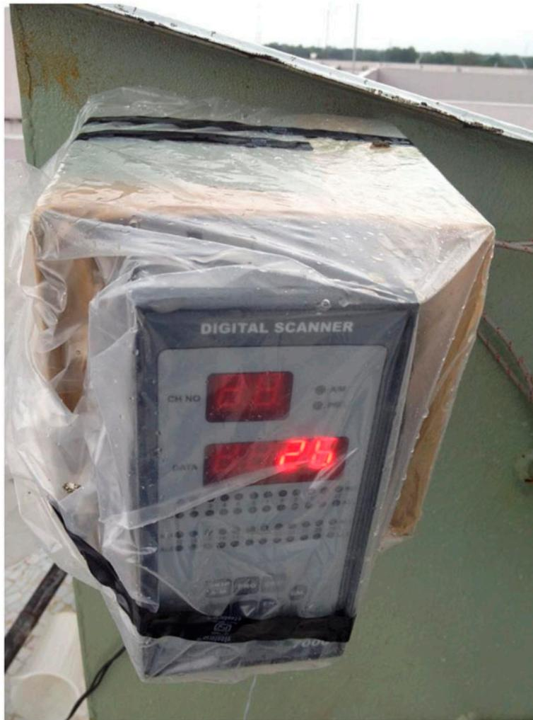
Fig. 2. Data logger attached to double-basin solar still with vacuum tubes.
