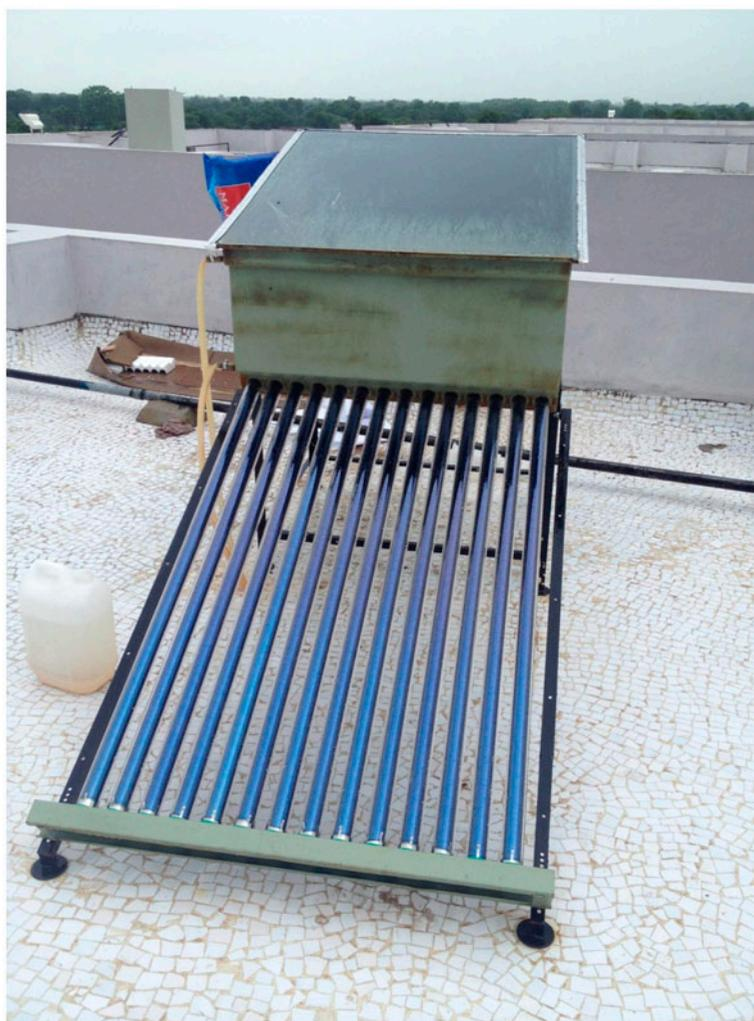
Fig. 1. Experimental set-up of double-basin solar still with vacuum tubes.
