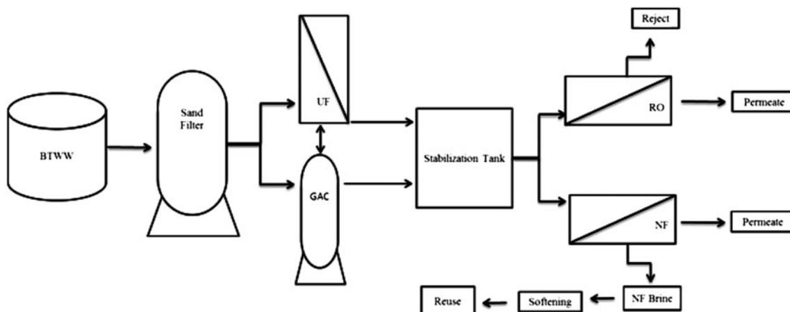
Fig. 1. Scheme of pilot membrane treatment system.
