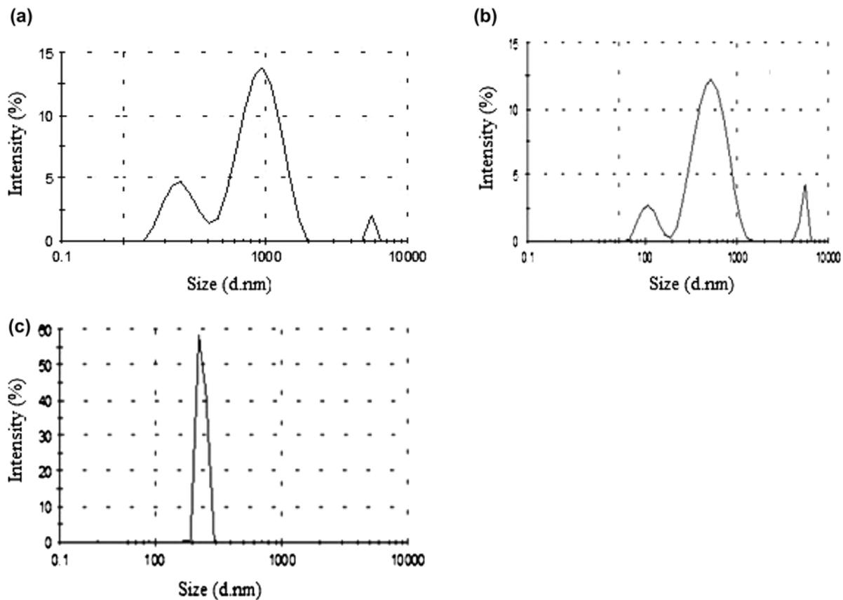
Fig. 2. PSD by intensity of: (a) biologically treated wastewater after sand filtration, (b) GAC adsorption, and (c) UF and GAC combined treatment systems (pH = 6.8 and conductivity = 6.9 mS cm<sup>-1</sup>).
