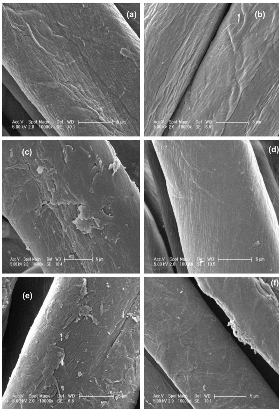
Fig. 6. SEM images of cotton fabric dyed with treated wastewaters: (a) process water, (b) NF permeate, (c) BTWW, (d) UF and GAC, (e) NF brine, and (f) softened NF brine 100%.
