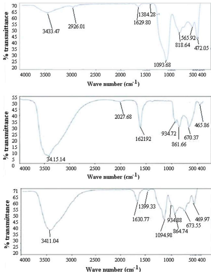
Fig. 3. FTIR Spectra of only PVC, NT, and PVC-based NT composite materials.
