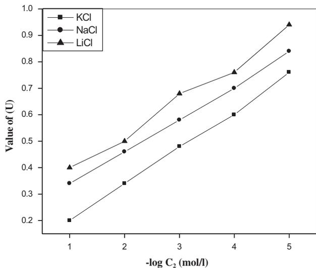
Fig. 9. The values of  $\bar{U}$  against the logarithm of various concentrations for PVC-based NT composite membrane.
