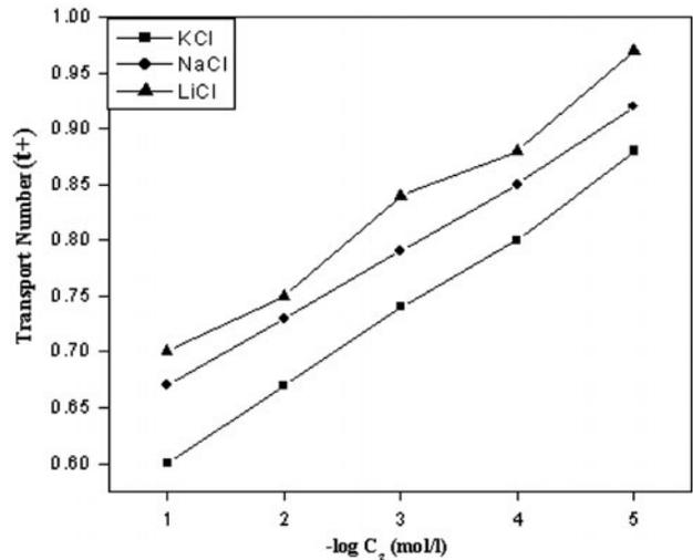
Fig. 8. Plot showing the transport number of PVC-based NT composite membrane for different used electrolytes.
