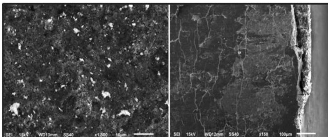
Fig. 2. SEM images of PVC-based NT composite membrane by two different magnifications.
