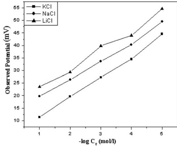
Fig. 5. Plots of observed membrane potentials against logarithm of concentration for PVC-based NT composite membrane.
