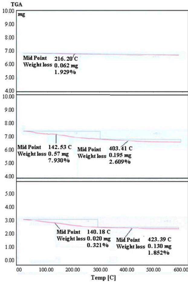
Fig. 4. TGA spectra of only PVC, NT, and PVC-based NT composite materials.
