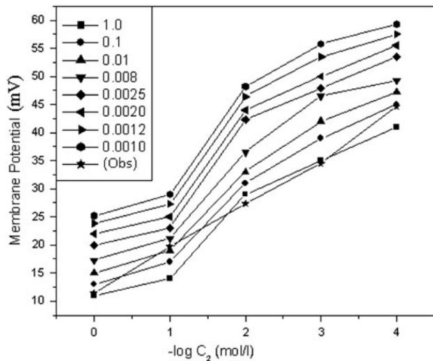
Fig. 6. Plots of theoretical and observed membrane potentials at different concentration of KCl, NaCl, and LiCl electrolyte solutions for PVC-based NT composite membrane.
