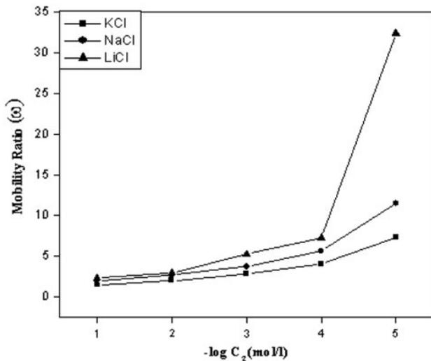
Fig. 7. The plot for mobility ratio of PVC-based NT composite membrane for different used electrolytes.
