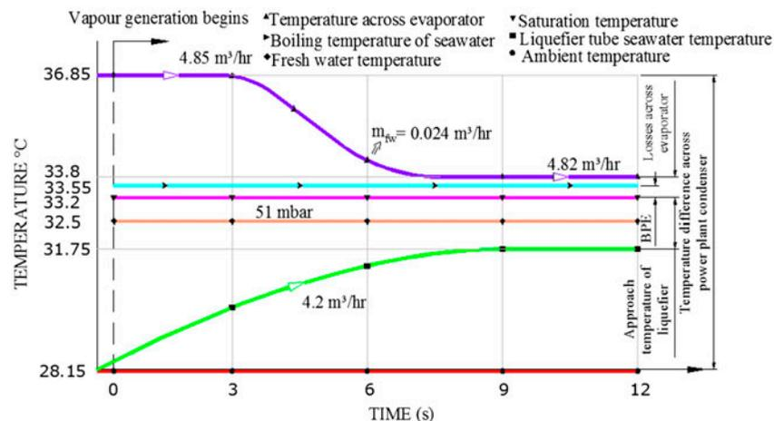
Fig. 4. Temperature profiles across plant components of evaporator and liquefier.
