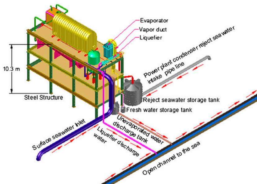
Fig. 2. CAD model of the proposed desalination plant.
