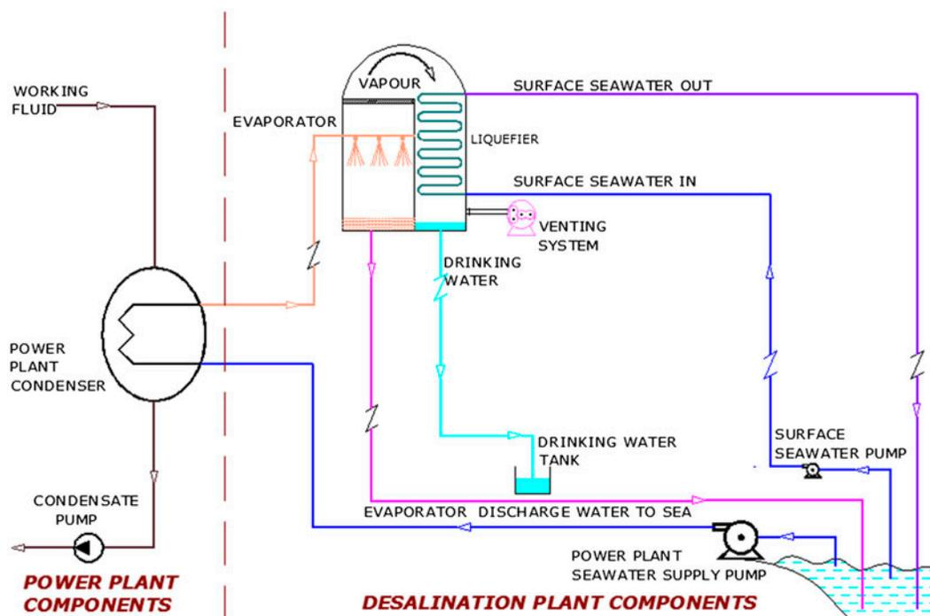
Fig. 1. Process scheme layout of the proposed desalination plant.
