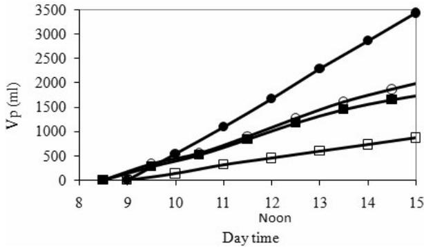
Fig. 4. Volume of produced water vs time. Feed water flow rate, ambient temperature and average irradiation are: ● 3 ml/s, 38°C, 822 W/m<sup>2</sup>; ○ 5 ml/s, 31°C, 839 W/m<sup>2</sup>; ■ 6 ml/s, 28°C, 790 W/m<sup>2</sup>; □ 11 ml/s, 34°C, 838 W/m<sup>2</sup>.
