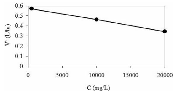
Fig. 9. Effect of feed water salinity, C, on the rate of water production, V'.
