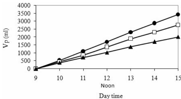
Fig. 8. Volume of water produced vs. time. Feed salinity, feed water flow rate, ambient temperature and average irradiation are: ● tap water, 3 ml/s, 38°C, 822 W/m<sup>2</sup>; □ 10,000 mg/L 4 ml/s, 36°C, 849 W/m<sup>2</sup>; ■ 20,000 mg/L, 2 ml/s, 41°C, 872 W/m<sup>2</sup>.
