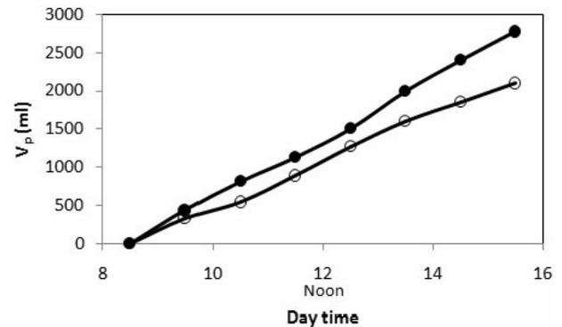
Fig. 7. Effect of cooling outer glass surface on volume of water produced vs. time. Feed water flow rate, ambient temperature and average irradiation are: ● 6 ml/s, 39°C, 767 W/m<sup>2</sup> (with cooling); ○ 7 ml/s, 39°C, 839 W/m<sup>2</sup> (without cooling).
