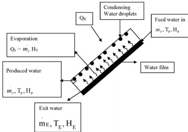
Fig. 3. Schematic diagram of the falling film for mass and energy balances.
