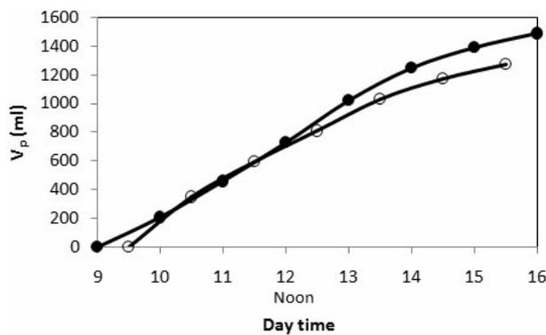
Fig. 6. Effect of the ambient temperature on the volume of produced water vs. time. Feed water flow rate, ambient temperature and average irradiation are: ● 9 ml/s, 28°C, 766 W/m<sup>2</sup>; ○ 10 ml/s, 19°C, 689 W/m<sup>2</sup>.
