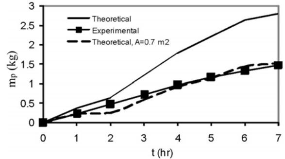
Fig. 12. Comparison of theoretically calculated and experimentally measured mass of water produced.
