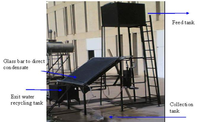
Fig. 1. Falling film solar desalination unit.
