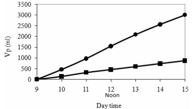
Fig. 5. Effect of feed water flow rate on amount of desalinated water vs. time. Feed water flow rate, ambient temperature and average irradiation were: ● 3 ml/s, 34°C, 883 W/m<sup>2</sup>; ■ 11 ml/s, 34°C, 838 W/m<sup>2</sup>.
