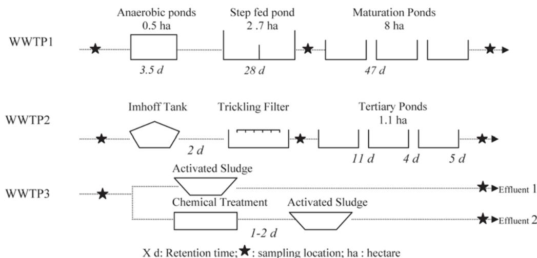
Fig. 1. Description of the three waste water treatment processes.
