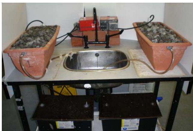
Fig. 1. Laboratory set-up for P-adsorption experiments.
