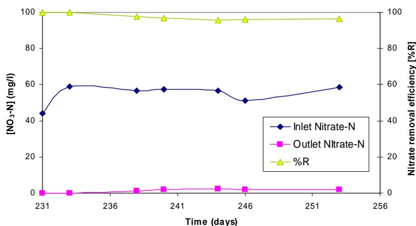
Fig. 2. Nitrate removal efficiencies and nitrate influent and effluent concentrations in the methanogenic/denitrifying reactor.
