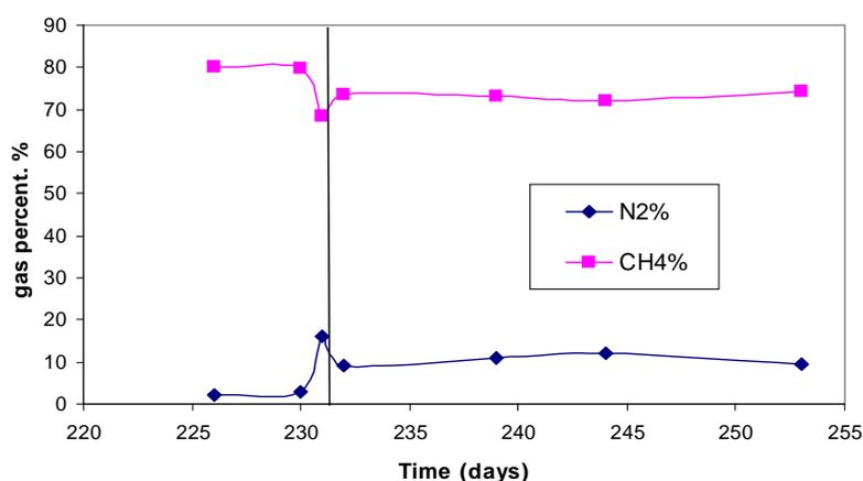
Fig. 4. Methane and nitrogen gas percentage in the gas collected from the UASB before and after the addition of nitrate to the feed. The separation line indicates the start of addition of nitrate to the feed.
