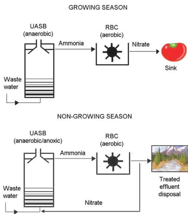
Fig. 1. Set up of the UASB–RBC treatment system in the growing season and in the non-growing season.
