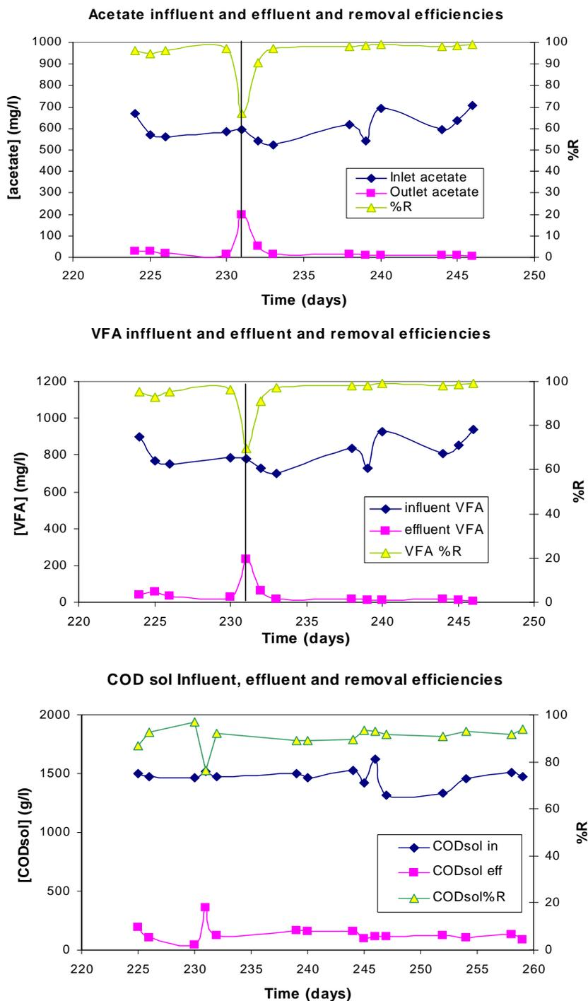
Fig. 3. Acetate, total VFA and  $\text{COD}_{\text{sol}}$  measured in the influent and effluent of the UASB and their corresponding removal efficiencies %R (expressed as a percentage of the influent concentration). The separation line indicates the start of addition of nitrate to the feed.
