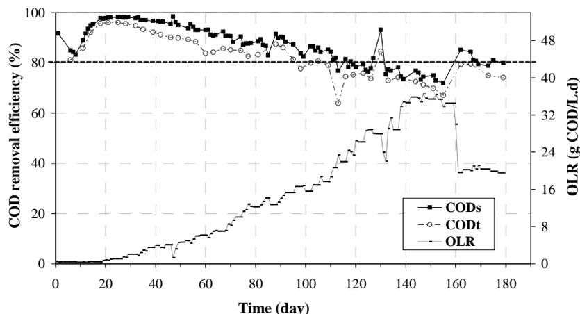
Fig. 2. Temporal variations of OLR and COD removal efficiencies for the reactor  $R_3$  treating winery wastewater.
