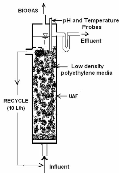
Fig. 1. Schematic diagram of a laboratory scale UAF.
