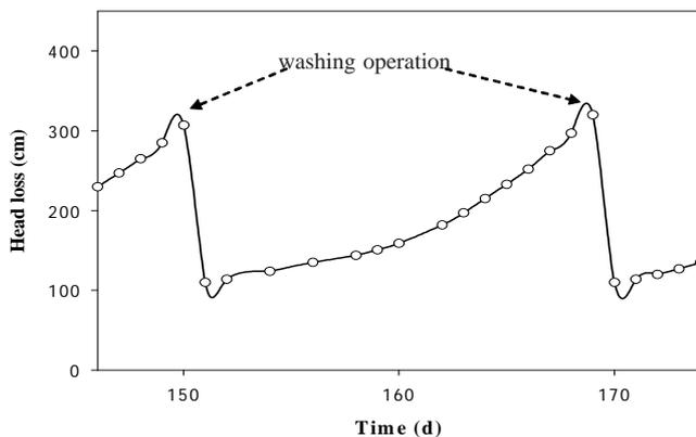
Fig. 5. Head loss profile recorded in period B during the interval between two washing operations.
