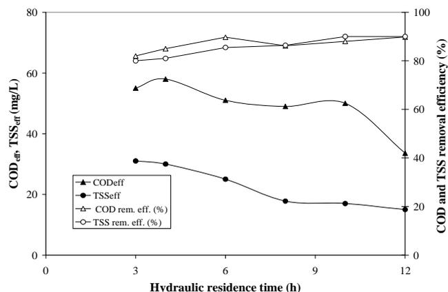
Fig. 3. COD and TSS concentrations in the effluent and their relative removal efficiencies as functions of hydraulic residence time during period B.
