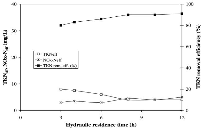
Fig. 4. TKN and  $\text{NO}_x\text{-N}$  concentrations in the effluent and TKN removal efficiencies as functions of hydraulic residence time during period B.
