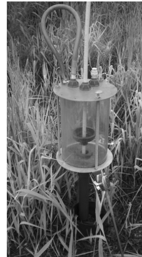
Fig. 3. Photograph of the experimental set-up at a Constructed Wetland in South Warwickshire, UK, depicting the Mariotte Siphon activated reservoir standing above the permeameter cell, which has been submersed into the gravel substrate.
