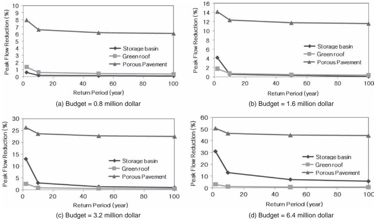
Fig. 4. Comparison of peak flow reduction by BMPs.
