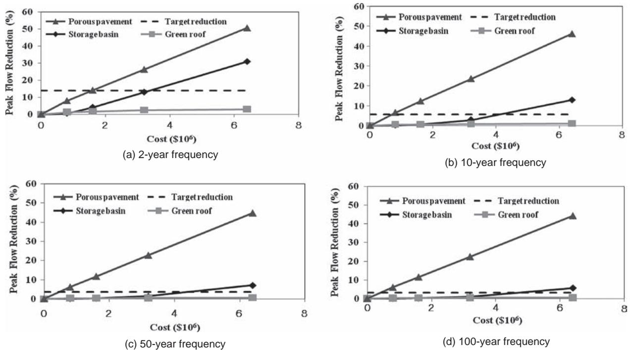
Fig. 3. Comparison of peak flow reduction by BMPs for the various budget ranges.
