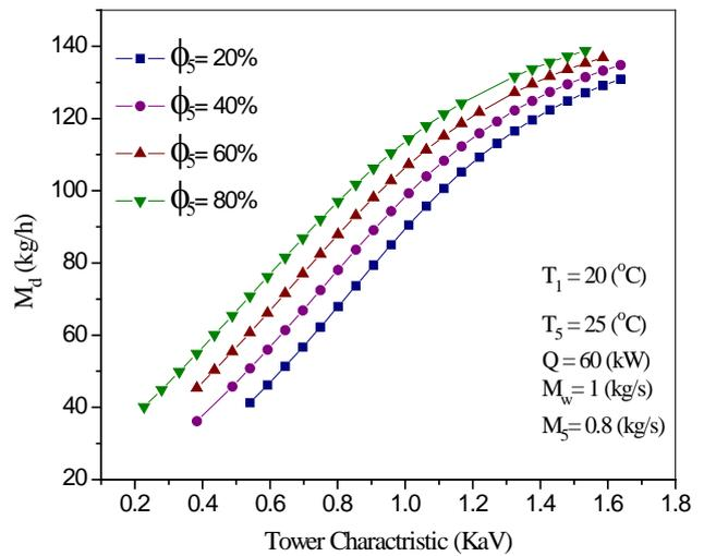
Fig. 8. Effect of humidifier characteristics ( $KaV$ ) on the fresh water production.
