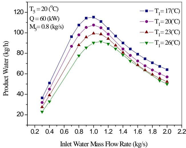
Fig. 6. Effect of inlet air flow rate on the fresh water production at different inlet air temperatures.
