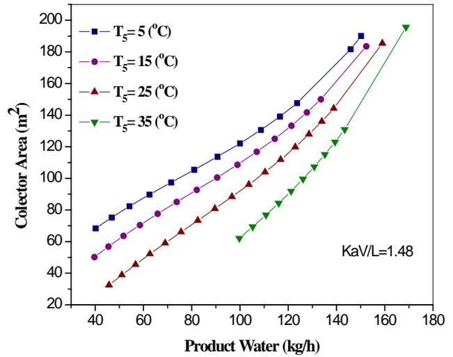
Fig. 10. Effect of solar collector area on the fresh water production.
