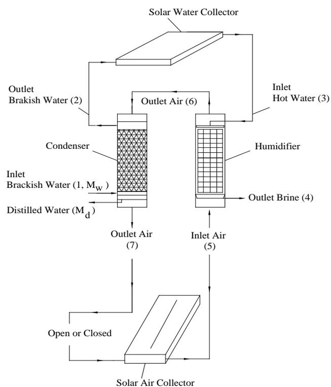
Fig. 1. Schematic of the plant.
