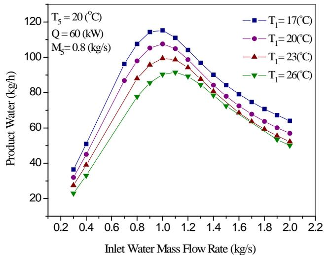
Fig. 5. Effect of brackish water flow rate on the fresh water production at different inlet water temperatures.
