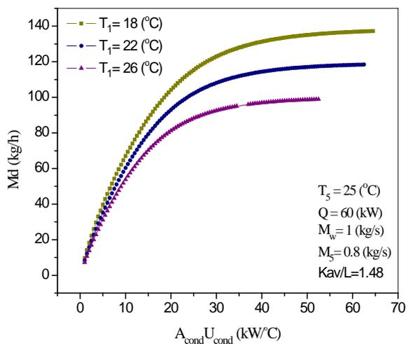
Fig. 7. Effect of condenser characteristics ( $AU$ ) on the fresh water production.
