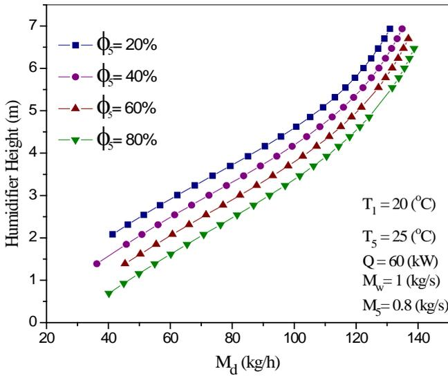
Fig. 9. Effect of humidifier height on the fresh water production.
