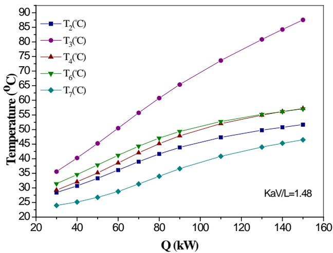
Fig. 11. Effect of heating input on the variation of temperature at the different components of the cycle.
