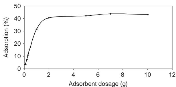
Fig. 3. Adsorption (%) - adsorbent dosage graph.
