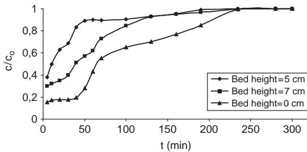
Fig. 7. Breakthrough curves for 5, 7 and 10 cm bed heights.
