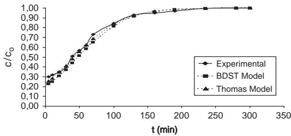
Fig. 8. Breakthrough curves after modelling of experimental data.
