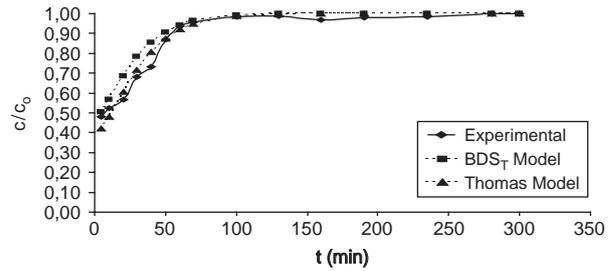
Fig. 10. Breakthrough curves after modelling of experimental data.
