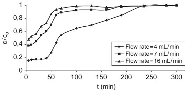
Fig. 9. Breakthrough curves for 4, 7 and 16 ml/min flow rates.
