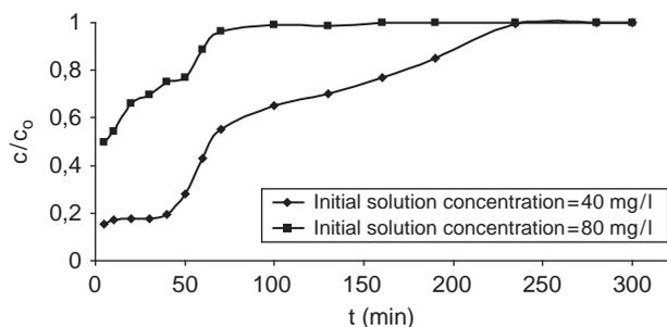
Fig. 11. Breakthrough curves for 40 and 80 mg/l initial solution concentrations.
