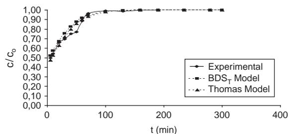
Fig. 12. Breakthrough curves after modelling of experimental data.
