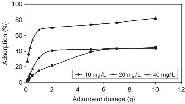
Fig. 4. Adsorption-adsorbent dosage graph for 10, 20 and 40 mg/l initial solution concentrations.
