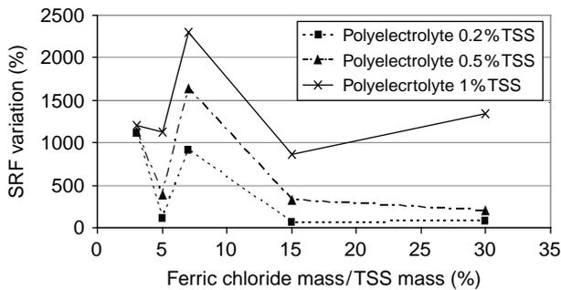
Fig. 1. SRF variation of MBRcfs due to conditioning: ferric chloride influence.
