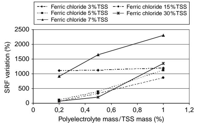
Fig. 2. SRF variation of MBRcfs due to conditioning: polyelectrolyte influence.
