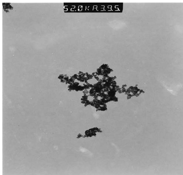
Fig. 2. TEM image of  $\text{Cd}_{0.97}\text{Co}_{0.03}\text{S}$  nanoparticles.
