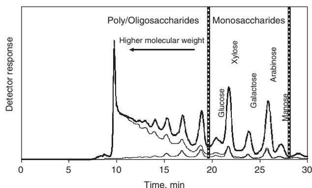
Fig. 2. Chromatographic elution pattern determined for (—) feed, (---) final retentate and (· · ·) final permeate obtained with the CARBOsep CHO 682 column.
