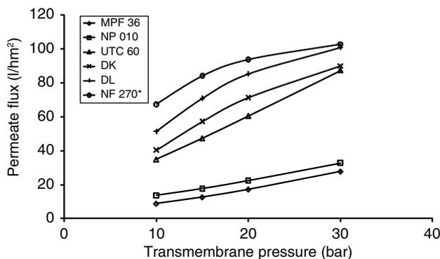
Fig. 4. Nanofiltration membrane behaviour in relationship of açai juice permeate flux (VRF = 1) using different transmembrane pressures (\*Means of three assays).
