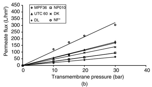
Fig. 3. Hydraulic permeability of nanofiltration membranes before (a) and after (b) tests with açai juice (\*Means of three assays).
