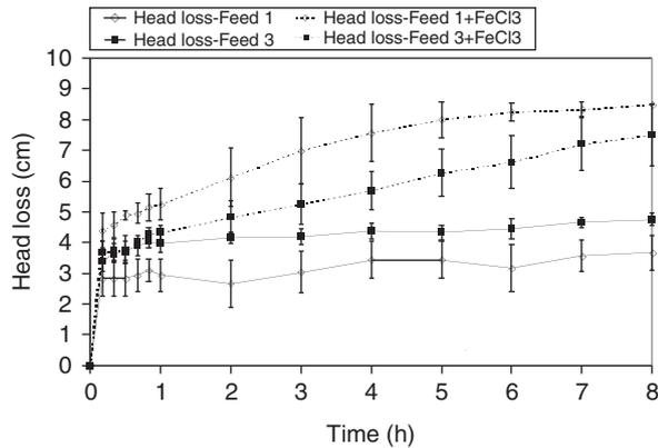
Fig. 6. Head loss development of DMF treating the types 1 and 3 feed with and without coagulation during the filtration cycle.
