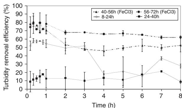
Fig. 5. Turbidity removal efficiency of DMF treating the type 3 feed with and without coagulation during various filtration periods (8–24, 24–40, 40–56 and 56–72 h).
