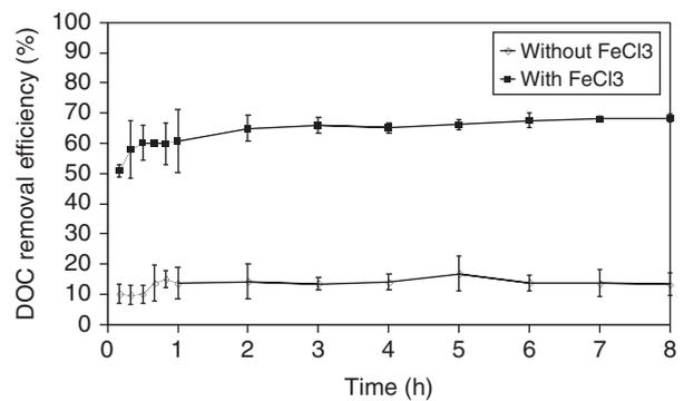
Fig. 8. DOC removal efficiency of DMF treating the type 4 feed.
