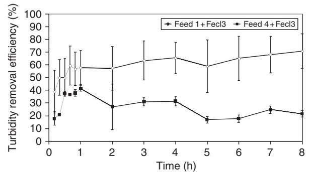
Fig. 7. Turbidity removal efficiency of DMF treating the types 1 and 4 feed with and without coagulation during the filtration cycle.
