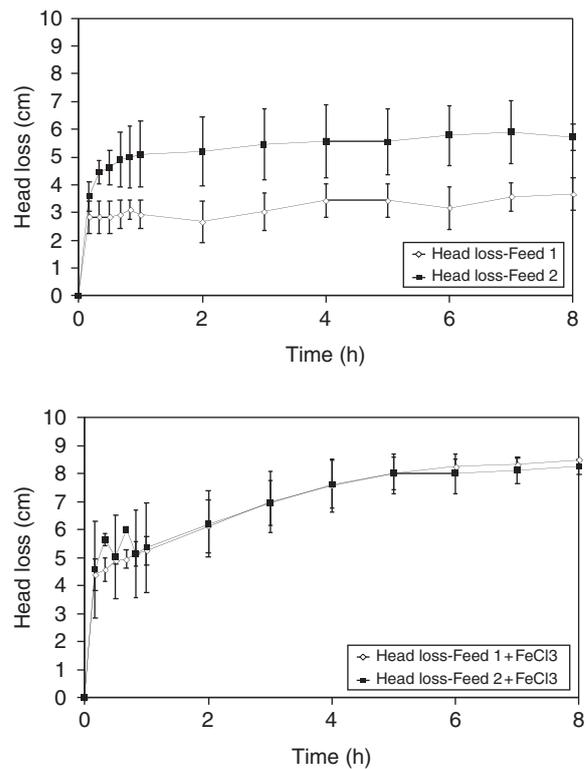
Fig. 3. Head loss development of DMF treating the types 1 and 2 feed with and without coagulation during the filtration cycle.
