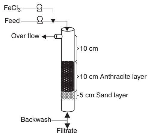
Fig. 1. Schematic of laboratory scale DMF.
