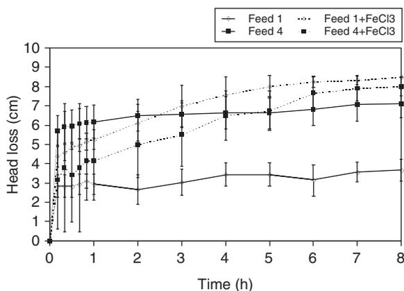
Fig. 9. Head loss development of DMF treating the types 1 and 4 feed with and without coagulation during the filtration cycle.
