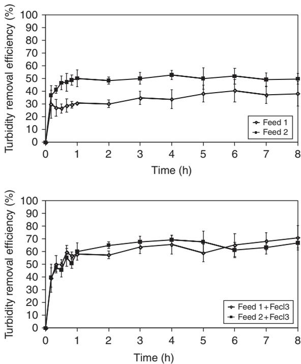
Fig. 2. Turbidity removal efficiency of DMF treating the types 1 and 2 feed with and without coagulation during the filtration cycle.
