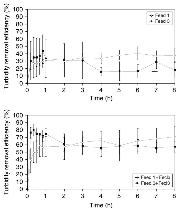
Fig. 4. Turbidity removal efficiency of DMF treating the types 1 and 3 feed with and without coagulation during the filtration cycle.
