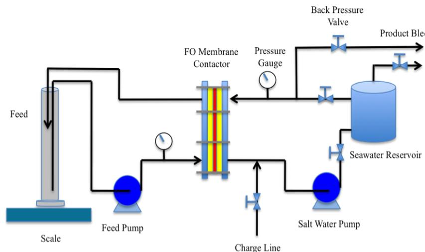
Fig. 1. PRO\TT flow diagram.
