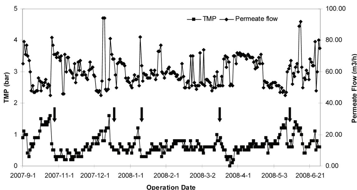
Fig. 3. Trans-membrane pressure and permeate flow of the UF units. The arrow ( $\downarrow$ ) indicates a chemical cleaning.
