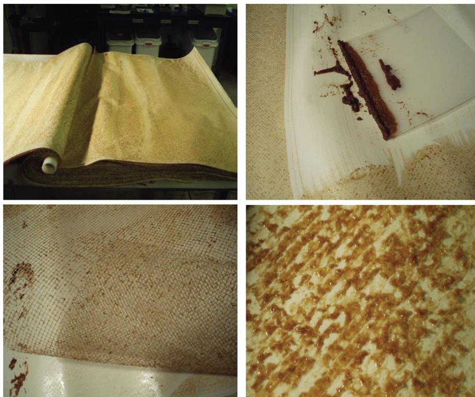
Fig. 7. Photos of the fouled membrane surface.
