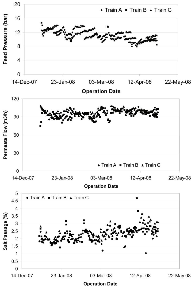
Fig. 4. Feed pressure, permeate flow, and salt passage of the three RO trains vs. operation time.
