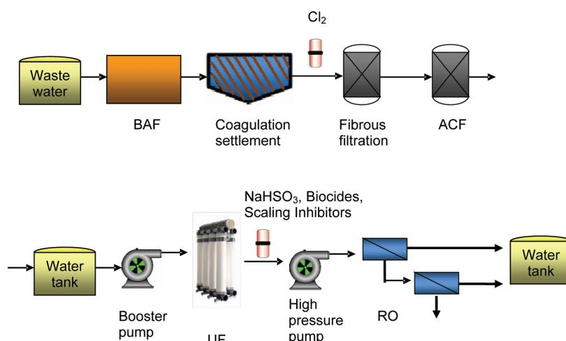
Fig. 1. Flowchart of the refinery wastewater reuse process.
