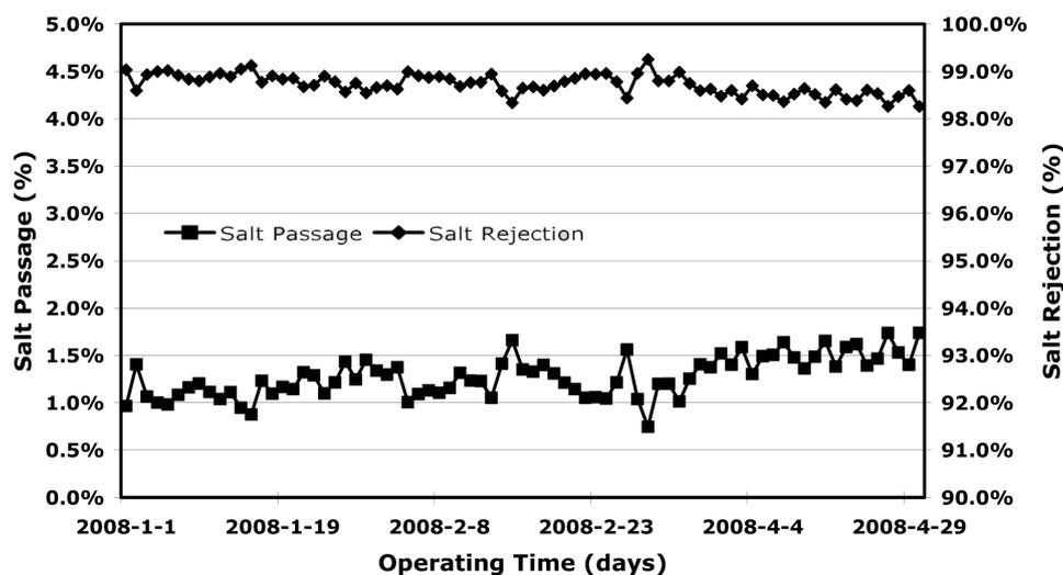
Fig. 5. Normalized salt passage of RO A vs. operation time.
