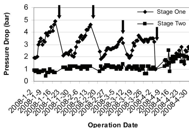
Fig. 6. Pressure drops of RO train C vs. operation time.
